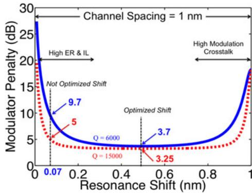
Fig. 9. Estimated modulator penalty for a channel spacing of 1 nm and different resonance shifts. If the shift of the resonance is small, then the IL and ER penalty are high. On the other hand, if the shift is too big, then the crosstalk penalty is very high. The optimum shift is about half of the channel spacing.
