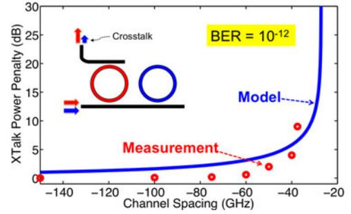
Fig. 8. Comparison of measured crosstalk power penalties (circles) and model (solid line) for two cascaded ring resonators at a bit error rate of  $10^{-12}$ . For channel spacings larger than 1 nm ( $\sim 120$  GHz), the penalty is negligible. However, penalty sharply increases as the channel spacing is reduced to below 40 GHz. Measurement data are taken from [66].
