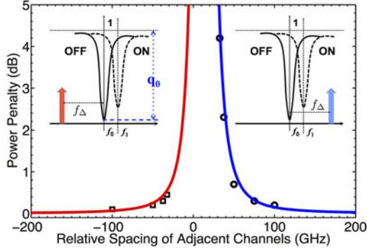
Fig. 4.  $PP_{\text{Mod-Xtalk}}$  (see Eq. (11)) for two cases: (blue) when the adjacent channel is at a higher frequency ( $f_{\Delta} > 0$ ), (red) when the adjacent channel is at a lower frequency ( $f_{\Delta} < 0$ ). Due to the unilateral shift of the ring modulator, the first case exhibits higher penalty than the second case. Measurement data [86] are denoted by circles and squares.
