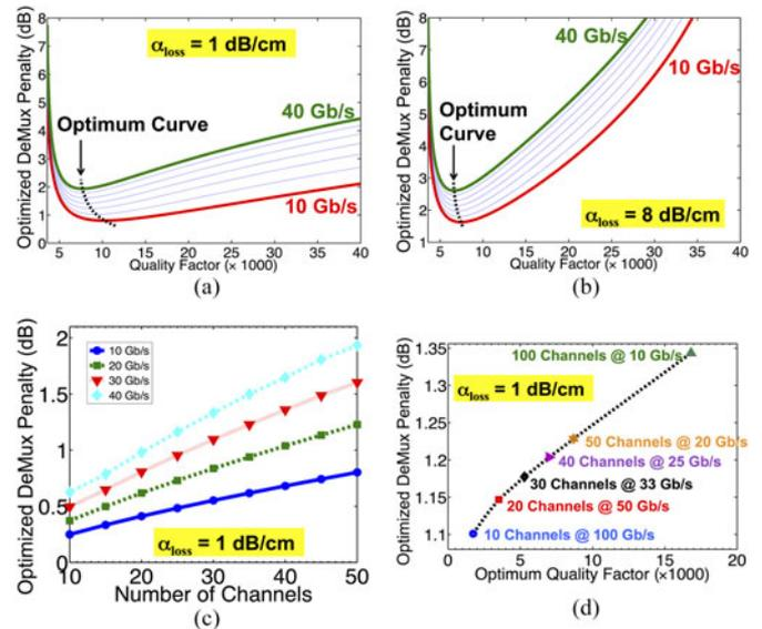
Fig. 10. Optimizing the penalty of demux ring filters by including the IL as a function of  $Q$ -factor of the ring. (a) Loss factor of the ring is 1 dB/cm and 50 channels. (b) Loss factor of the ring is 8 dB/cm and 50 channels. (c) Power penalty for different number of channels and bit rates (loss = 1 dB/cm) when using demux rings with optimized  $Q$ . (d) Optimum penalty and its corresponding  $Q$ -factor for an aggregate rate of 1 Tb/s and different channel rates (loss = 1 dB/cm).
