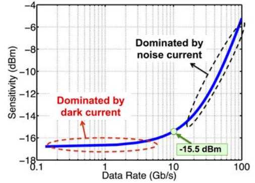
Fig. 12. Estimated sensitivity of the receiver as a function of the modulation data rate. At low data rates, dark current dominates over the noise current and thus the sensitivity is almost constant, whereas at high data rates the noise current dominates over the dark current and sensitivity is reduced.
