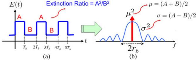
Fig. 2. Envelope electric field of the (a) NRZ-OOK modulation, and its (b) power spectral density. ER is the ratio of the optical power of the high level to the optical power of the low level of the electric field.
