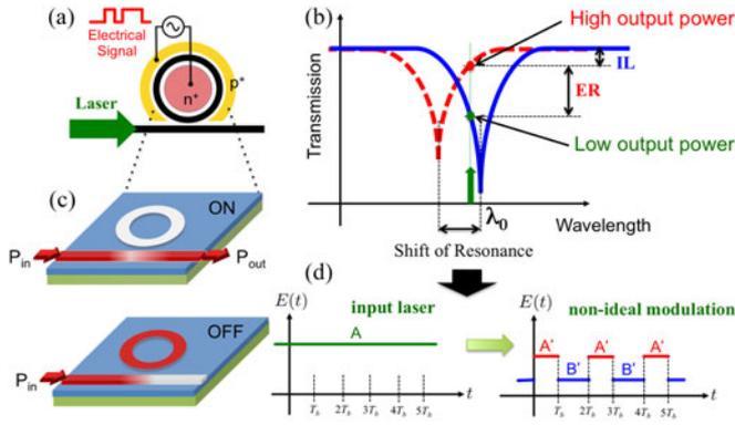
Fig. 3. (a) Schematic view of a microring modulator. The high-speed electrical signal is applied to the p-n-junction embedded inside the silicon ring. (b) Modulation of the input laser by shifting the resonance of the ring to create high and low levels of optical power at the output. (c) Graphical view of how ON and OFF states of the light at the output happen. (d) Time-domain presentation of a non-ideal NRZ OOK modulation.
