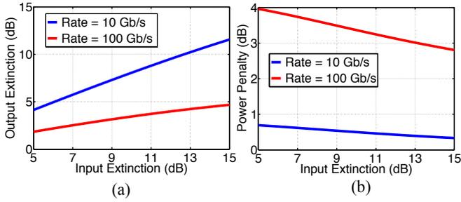
Fig. 2. (a) Calculation of the output extinction ratio (in dB) as a function of the input extinction ratio (in dB) for 10 Gb/s (blue) and 100 Gb/s (red) data rate. (b) Power penalty as a function of the input extinction ratio for 10 Gb/s and 100 Gb/s.
