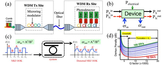
Fig. 1. (a) Schematic of a chip-to-chip MRR-based silicon photonic link. (b) High-level modeling of an optical device along the link. (c) Effect of the narrow bandwidth of the demux ring on the extinction ratio of modulation. (d) Calculation of the total demux penalty for various  $Q$ -factor and bit rates.
