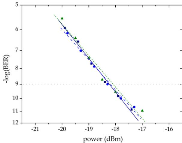
**Fig. 3.** BER plots recorded at the drop port showing no observable power penalty due to wavelength crosstalk; 16 (■, solid line), 12 (●, long-dashed line), and 1 (▲, short-dashed line) wavelength channel.
