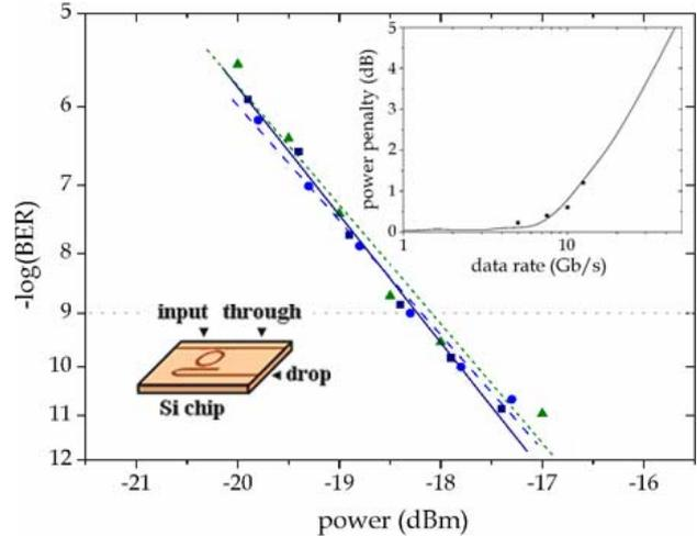
**Fig. 2.** BER plots recorded at the drop port for 16 (■, solid line), 12 (●, long-dashed line), and 1 (▲, short-dashed line) signals; measured (■) and simulated (line) single-channel power penalty of the drop port versus data rate (right inset); switch layout (left inset).
