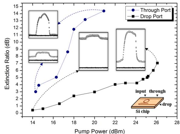
Figure 2: Measured extinction ratios with varying pump power for through (●) and drop (■) ports with insets of corresponding extinction ratios (using a 16-point average) and device layout.
