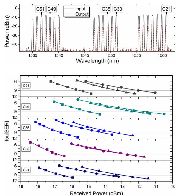
Figure 1: (top) WDM signal input/output spectra at drop port. (bottom) BER curves for through (▲), drop (●), and reference (■) ports for five of 20 channels.
