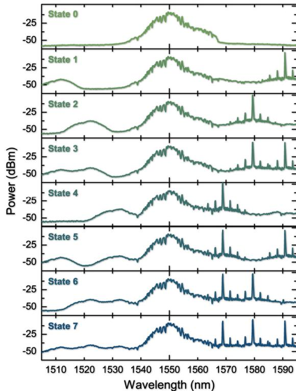
**Fig. 2:** Output spectra for the resulting signal egressing from the chip for each possible state of the  $3 \times 320$ -Gb/s wavelength multicast. The CW wavelength channels are centered at 1568.8, 1579.4, and 1590.8 nm, the pump signal is centered at 1550 nm, producing wavelength-multicasted wavelength channels centered at 1511.8, 1522.0, and 1532.2 nm. The OSNR in the spectra is limited by the dynamic range of the OSA.
