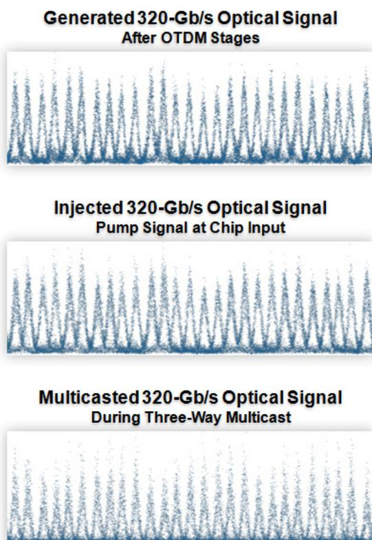
**Fig. 4:** Eye diagrams of the generated, injected, and wavelength-multicasted (centered at 1532.2 nm) optical signal during the  $3 \times 320$ -Gb/s wavelength multicast. Here, the pulse separation is 3.125 ps.
