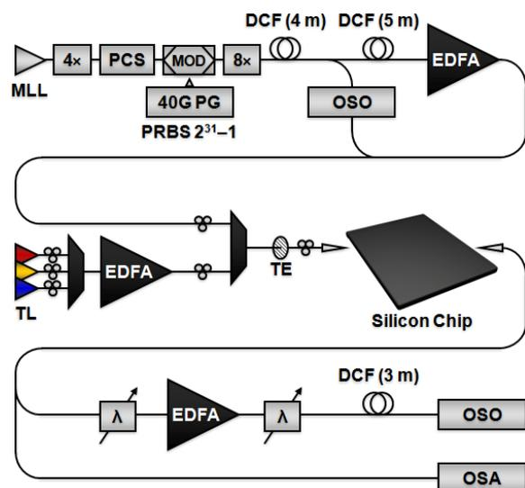
**Fig. 1:** Diagram of experimental setup used for the 3×320-Gb/s wavelength multicast.
