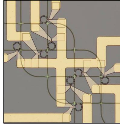
Fig. 4 Microscope image of the fabricated non-blocking four-port bidirectional multi-wavelength message router.
