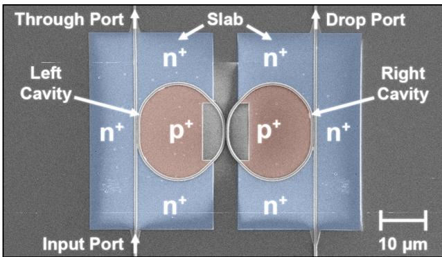
Fig. 3 Top-view scanning-electron-microscope (SEM) image of the silicon microring resonator electro-optic switch.
