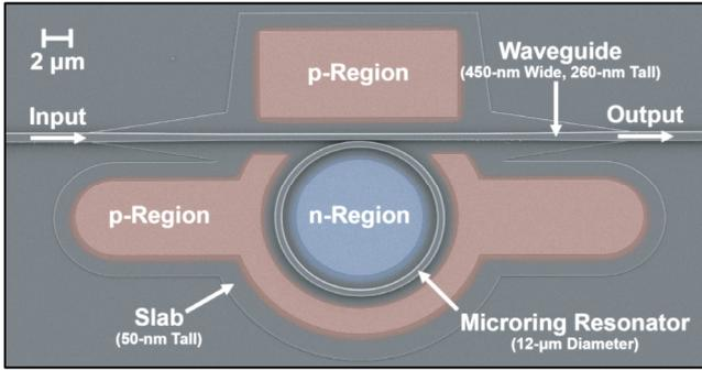
Fig. 2 Top-view scanning-electron-microscope (SEM) image of the silicon microring resonator electro-optic modulator.
