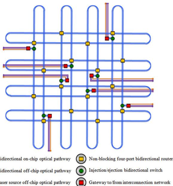
Fig. 1 Topology of the eight-port non-blocking torus nanophotonic NoC, with corresponding optical pathways and nanophotonic network elements.
