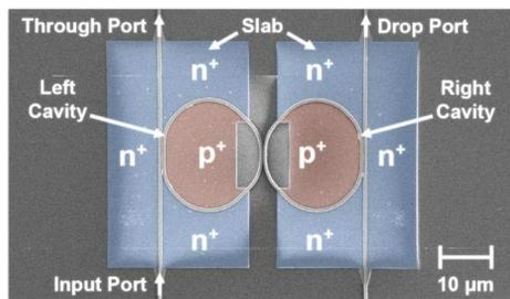
Fig. 2. Top-view scanning-electron-microscope (SEM) image of the silicon photonic microring resonator electrooptic switch.
