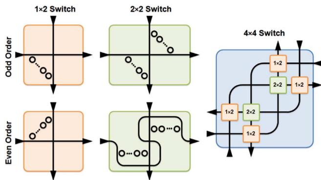
Fig. 1. Elementary models for  $1 \times 2$  and  $2 \times 2$  switching building blocks, implemented with both odd- and even-order microring resonators (left), as well as the nonblocking  $4 \times 4$  switch constructed using these models (right).
