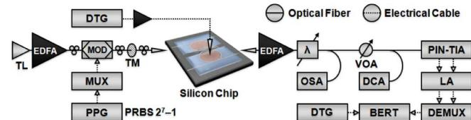
Fig. 3. Diagram of the experimental setup used for spectral and temporal evaluations, as well as BER and power penalty characterizations, using the silicon photonic microring resonator electrooptic second-order  $1 \times 2$  switch.
