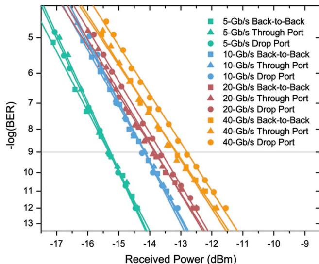
Fig. 7. Experimentally measured BER curves for packetized optical signals with 5-, 10-, 20-, and 40-Gb/s data rates, egressing from both output ports of the silicon photonic microring resonator electrooptic switch, as well bypassing the silicon chip in the back-to-back case.
