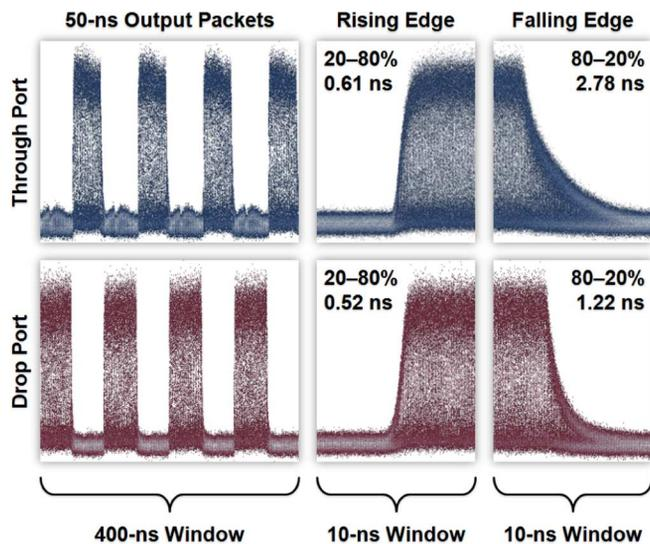
Fig. 6. Output optical packets encoded with 40-Gb/s data for both output ports of the silicon photonic microring resonator electrooptic switch in the active state, with rising and falling edges.
