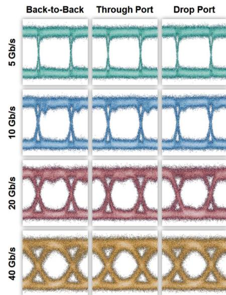
Fig. 5. Output eye diagrams for optical signals with 5-, 10-, 20-, and 40-Gb/s data rates, egressing from both output ports of the silicon photonic microring resonator electrooptic switch, as well as bypassing the silicon chip in the back-to-back case.
