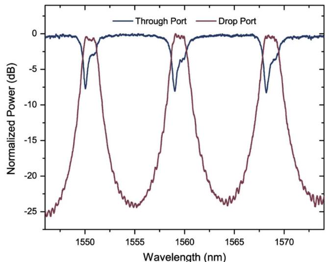
Fig. 4. Spectra of the silicon photonic microring resonator electrooptic switch for both output ports in the passive state.
