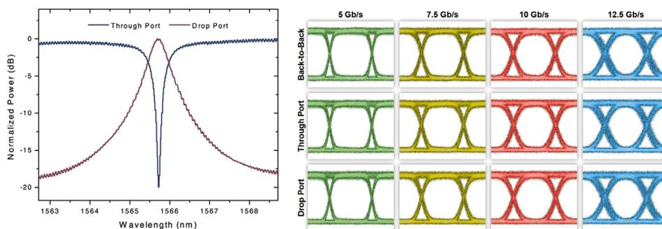
Fig. 2. Spectral response of the multi-layer silicon photonic microring resonator filter for both output ports (left), and output eye diagrams for optical signals with 5-, 7.5-, 10-, and 12.5-Gb/s data rates, egressing from both output ports of the filter, as well bypassing the silicon chip in the back-to-back case (right).
