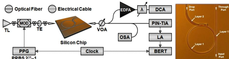
Fig. 1. Diagram of the experimental setup used for BER measurements using the multi-layer silicon photonic microring resonator filter (left), and top-view microscope image of the device (right).
