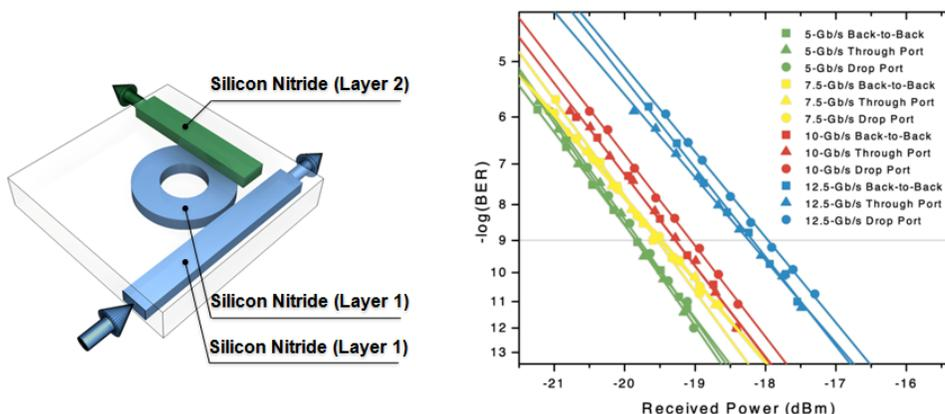
Fig. 3. Three-dimensional schematic representation of the multi-layer silicon photonic microring resonator filter (left), and measured BER curves for optical signals with 5-, 7.5-, 10-, and 12.5-Gb/s data rates, egressing from both output ports of the filter, as well as bypassing the silicon chip in the back-to-back case (right).
