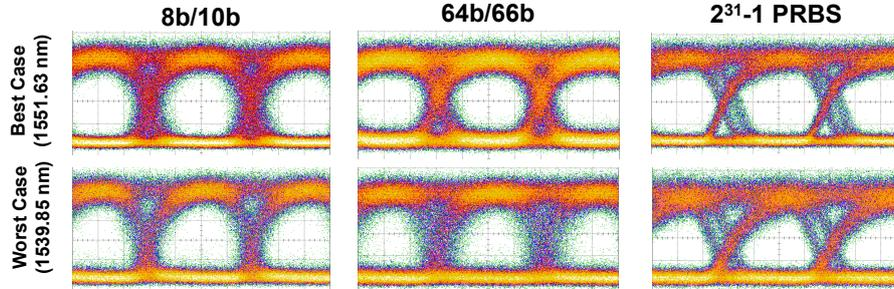
**Fig. 4:** Optical eye diagrams of the 4×2.5-Gb/s wavelength channels showing microring-modulated modulated 8b/10 and 64b/66b memory communication and  $2^{31}$ -1 PRBS (100 ps/div).
