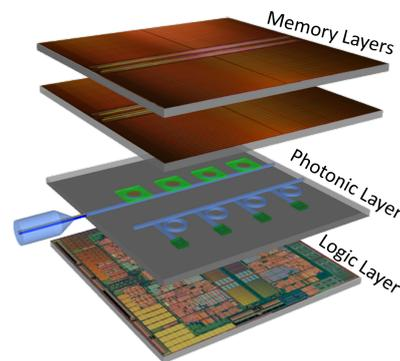
**Fig. 1:** Illustration of 3D-stacked OCM node. The high-speed logic layer interfaces with the memory layers to drive the photonic components.
