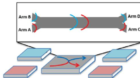
**Figure 1.** Data transmitted on Quasi-TM mode traverses from A to C and B to D, conceptually integrated into a multi-node system.
