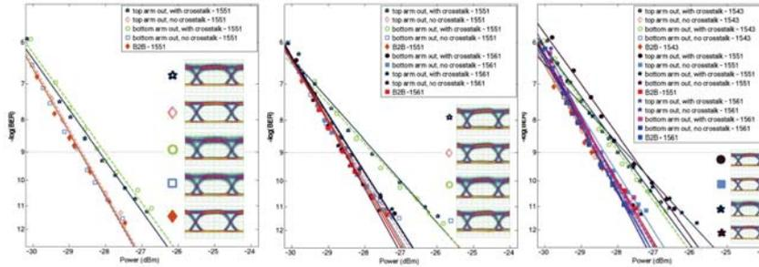
Figure 3. BER Measurement with 1 (left), 2 (middle), and 3 (right) operating wavelengths. Eye diagrams correspond to items at 1555 nm.
