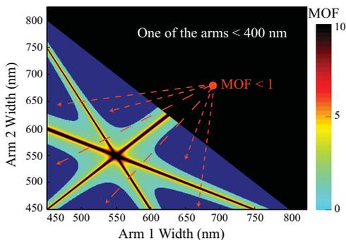
**Figure 4.** Asymmetric Y-junction design space according to (1) assuming  $\theta = 0.5$  degrees, a multimode interconnect width ( $w_{mm}$ ) of  $w_{mm} = 1.65 \mu\text{m}$ , and the width of arm 3 ( $w_{a3}$ ) is  $w_{a3} = w_{mm} - w_{a1} - w_{a2}$ . Blacked-out regions indicate a geometry that results in one arm width being  $< 400$  nm. Dark blue regions represent designs where  $\text{MOF} < 1$ , representing effective  $3 \times 3$  mode multiplexer designs.
