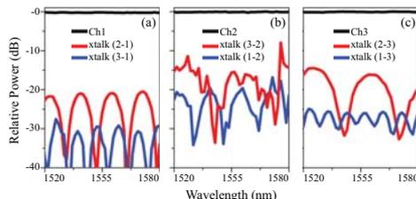
**Figure 5.** Image illustrates a theoretical spectral scan of a 3-mode device with 0.5 degree Y-junction angles simulated using the design methodology described in [5] with geometry  $250 \text{ nm} \times 450 \text{ nm}$  for arm 1,  $250 \text{ nm} \times 520 \text{ nm}$  for arm 2 and  $250 \times 680 \text{ nm}$  for arm 3. The interconnect cross section is  $250 \text{ nm} \times 1.6 \mu\text{m}$  and is 1 mm long.
