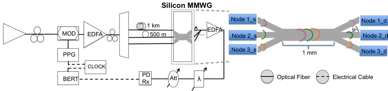
Fig. 1. Experimental setup, the integrated waveguide supporting 3 modes simultaneously, with data being transmitted on-chip along the Quasi-TM mode from Node1\_s to Node1\_d, Node2\_s to Node2\_d, and Node3\_s to Node3\_d, with indices denoting source and destination.
