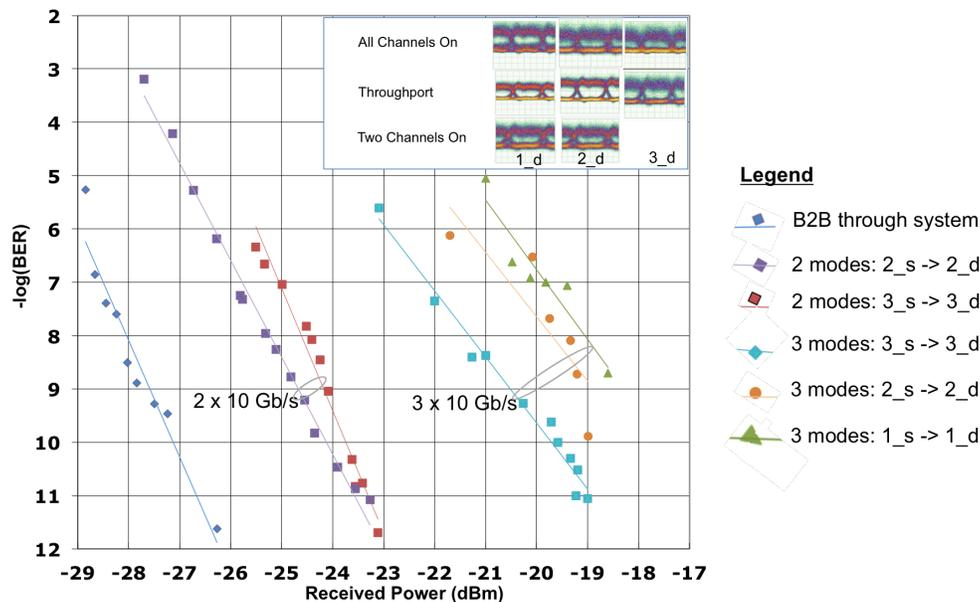
Fig. 2. BER measurement with two arms (1\_s and 2\_s) and three arms transmitting 10 Gb/s data simultaneously. Eye diagrams taken at the 3 channels (vert.) featuring labeled characteristics (horiz.).
