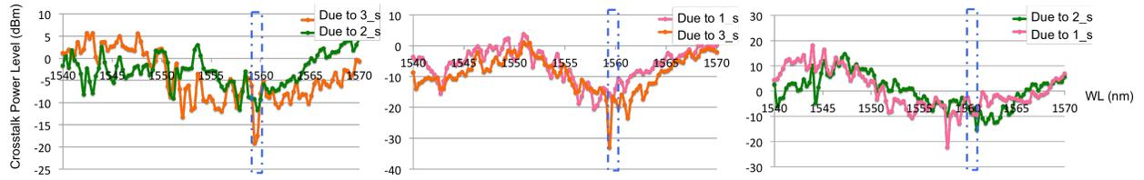
Fig. 3. Graphs of crosstalk level at 1\_d, 2\_d, and 3\_d channels of the waveguide across varying wavelengths due to combinations of 1\_s, 2\_s, and 3\_s. Dashed line indicates region selected for best crosstalk levels across all 3 channels.
