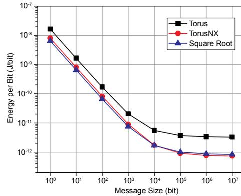
Figure 6. Transmission efficiency of the photonic topologies.
