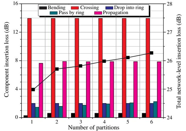
Fig. 9. (Color online) Insertion loss analysis of the TorusNX topology for varying levels of partitioning. Column plots correspond to worst-case insertion loss per component among all possible network paths (left-vertical axis). The line plot corresponds to the greatest total network-level insertion loss path among all possible network paths (right-vertical axis). The lossiest path does not necessarily correspond with the sum of the worst-case losses per component.
