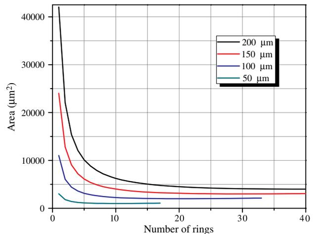
Fig. 10. (Color online) Photonic router footprint for varying number of rings (which corresponds to the number of WDM partitions enabled by the router). Legend indicates the ring diameter for the single-ring case.
