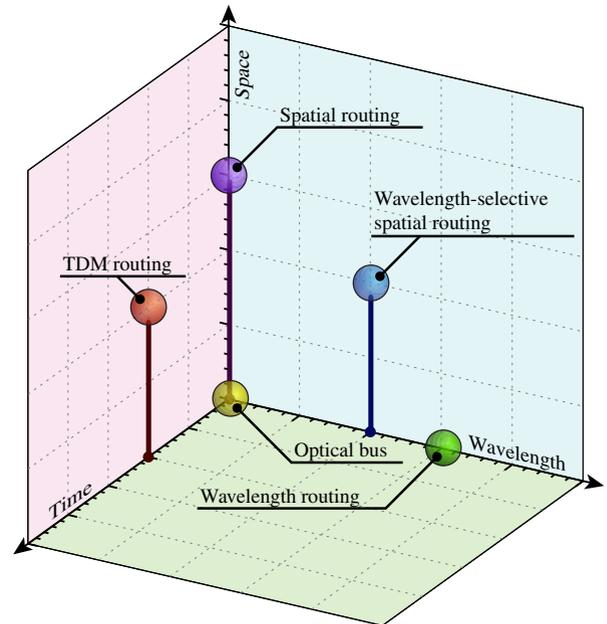
Fig. 2. (Color online) Routing technique design space based on three arbitration domains: time, wavelength, and space.
