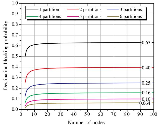
Fig. 11. (Color online) Destination blocking probability in a non-blocking network for varying number of interleaved channels. The limit of each blocking probability as  $N \rightarrow \infty$  is superimposed on the right of the plot.
