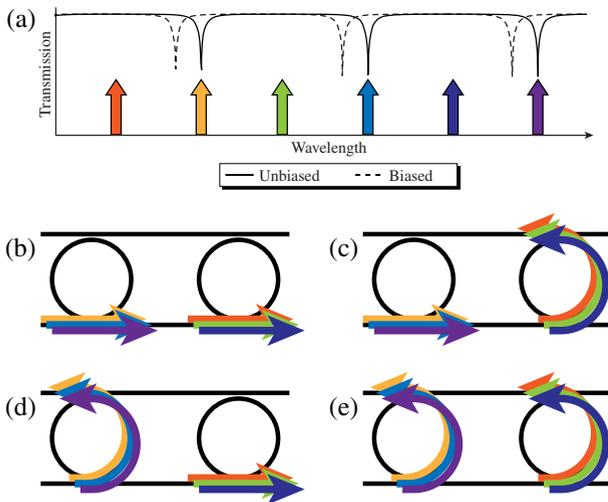
Fig. 3. (Color online) (a) Spectral placement of two WDM partitions (each containing three wavelength channels), with respect to the spectrum of an electro-optic broadband ring switch. (b)–(e) Four possible routing configurations for a two-partition router.
