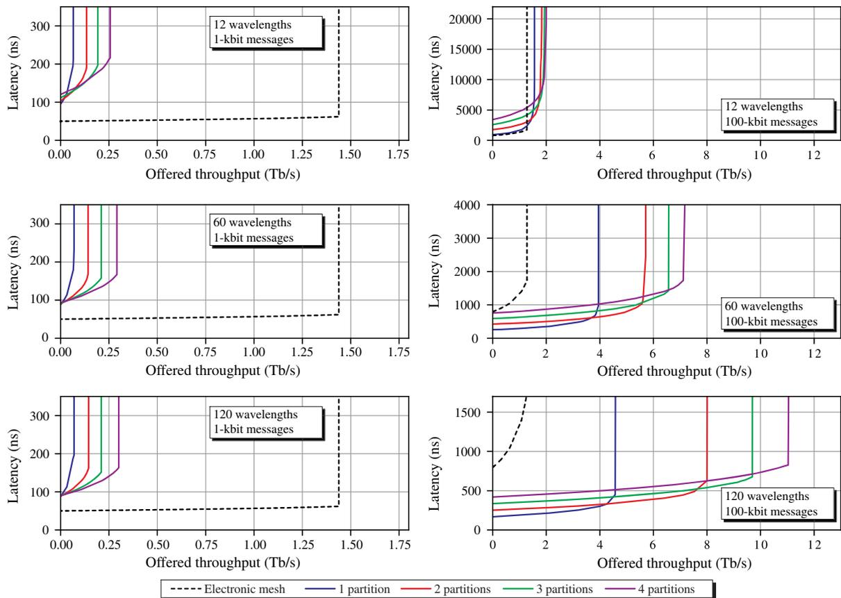
Fig. 12. (Color online) Average latency versus offered throughput for varying number of WDM partitions, message sizes, and number of wavelength channels. Electronic mesh performance is shown as a dotted line.
