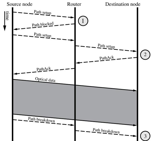
Fig. 5. Example timing diagram of the circuit-switching and WSSR allocation protocol. A path provisioning request is initially blocked, but is successful upon re-attempt.
