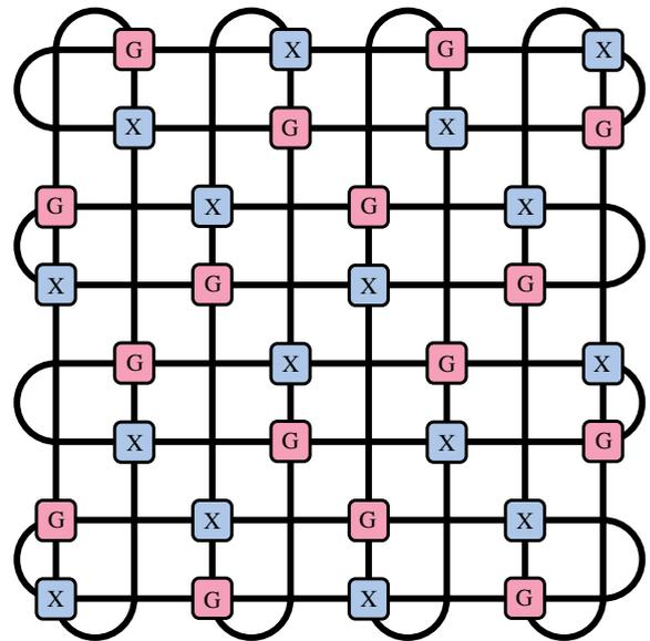
Fig. 7. (Color online) Schematic of the TorusNX topology. ‘G’ blocks represent gateway photonic switches and ‘X’ blocks represent  $4 \times 4$  non-blocking photonic switches. Lines indicate bidirectional links which are composed of two waveguides that are used for counter-propagating lightwaves.
