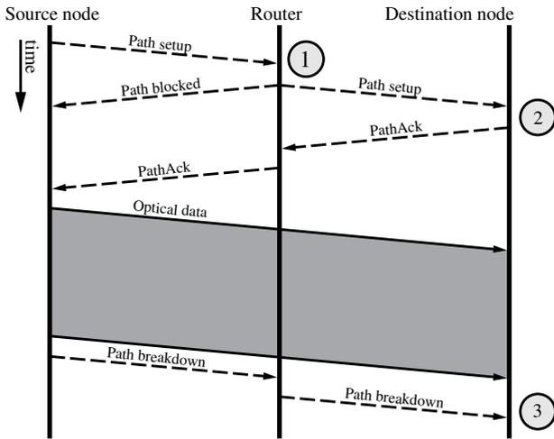
Fig. 6. Example timing diagram of the WSSR allocation protocol. If a single path provisioning request is attempted with multiple partitions, a path setup request can partially block on a particular partition while being successful on another partition.
