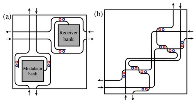
Fig. 8. (Color online) Schematic of the TorusNX photonic routers configured with two WDM partitions: (a) gateway switch and (b)  $4 \times 4$  non-blocking photonic switch.
