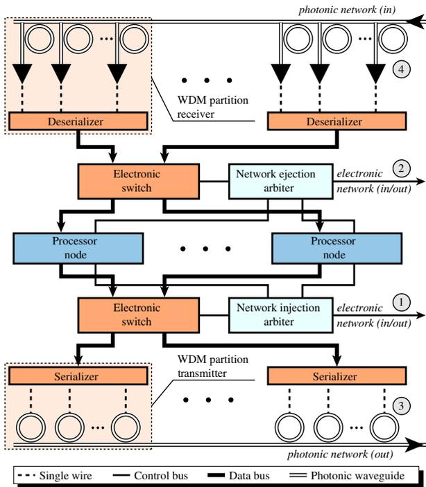
Fig. 4. (Color online) The WSSR gateway architecture with concentrating processing cores.
