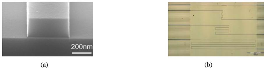
Fig.1 Silicon photonic wire waveguides: (a) cross-section view and (b) overhead view with 1 mm scale.
