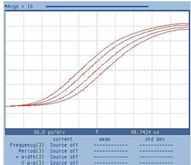
Figure 7. Opto-electronic Transmitter - 20ps Edge Placement Resolution
