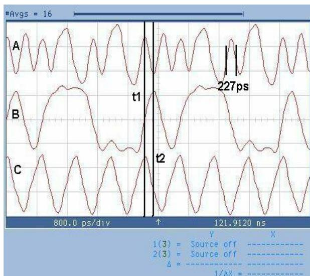
Figure 11. Demonstration of 4.4Gbps Output (A)
