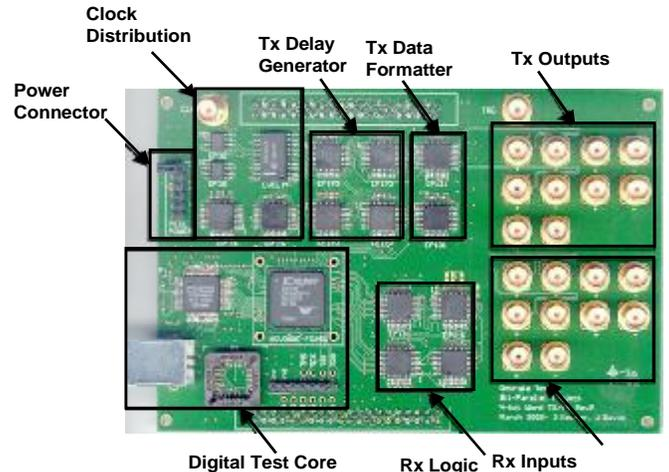
Figure 4. Multi-gigahertz Tx/Rx Photograph [2].
