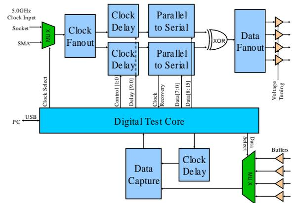
Figure 10. Nano-scale wafer-prober - Block Diagram
