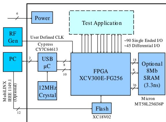
Figure 1. Digital Test Core Block Diagram.
