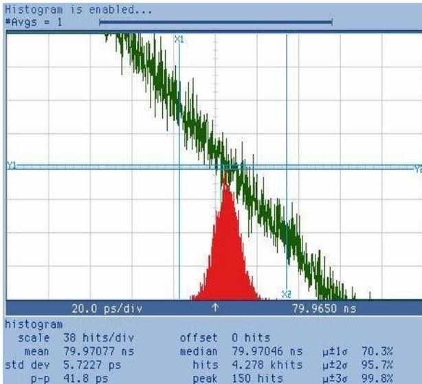
Figure 8. Opto-electronic Transmitter – Jitter Measurements
