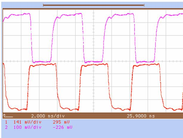
Figure 9. Electrical/Optical Conversion
