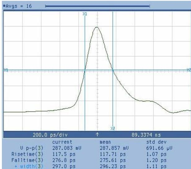
Figure 6. Opto-electronic Transmitter - Minimum Pulse Width (<300ps)
