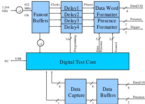
Figure 3. Opto-electronic Tx/Rx Block Diagram.
