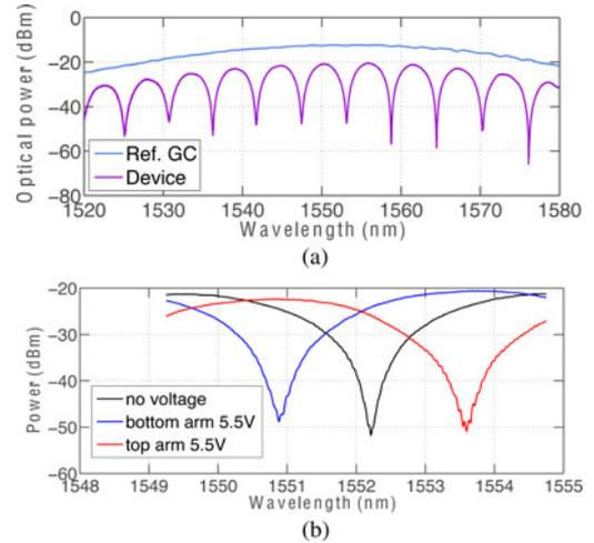
Fig. 5. (a) Optical spectra: device versus reference grating coupler (GC). (b)  $\pi$  phase shift under 5.5 V voltage on each arm.
