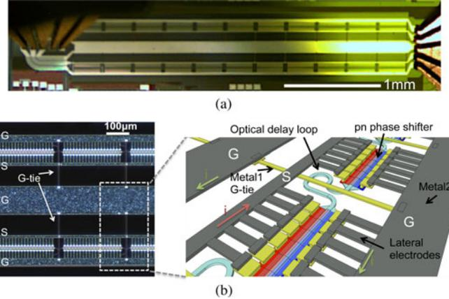
Fig. 3. (a) Fabricated device under probed testing: GSGSG probe on the right is for driving, and GSGSG probe on the left is for providing  $50\text{-}\Omega$  termination to each device arm, and (b) microphotograph of a section of the device, mainly top metal (Metal2) is visible. Inset (not-to-scale): details near a ground-plane lateral connection (G-tie) and the optical delay loop for re-aligning optical and RF phase.
