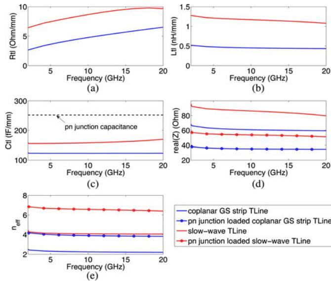
Fig. 2. Comparison of simulated transmission line parameters. Coplanar GS strip line parameters:  $g = 50\mu\text{m}$ ,  $s = 50\mu\text{m}$ , and  $d = 5\mu\text{m}$ . Slow-wave transmission line parameters:  $g = 30\mu\text{m}$ ,  $s = 10\mu\text{m}$ ,  $d = 6\mu\text{m}$ ,  $w = 5\mu\text{m}$ ,  $p = 14\mu\text{m}$  and  $D = 100\mu\text{m}$ .
