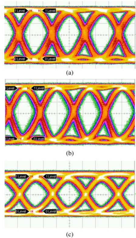
Fig. 8. Error-free ( $\text{BER} < 1e-12$ ) 40 Gb/s eye diagrams taken during the BER measurement: (a) Lithium Niobate modulator under  $5.4 V_{pp}$  drive. (b) Si TWMZ modulator under  $4.8 V_{pp}$  differential drive. (c) Si TWMZ modulator under  $1.6 V_{pp}$  differential drive.
