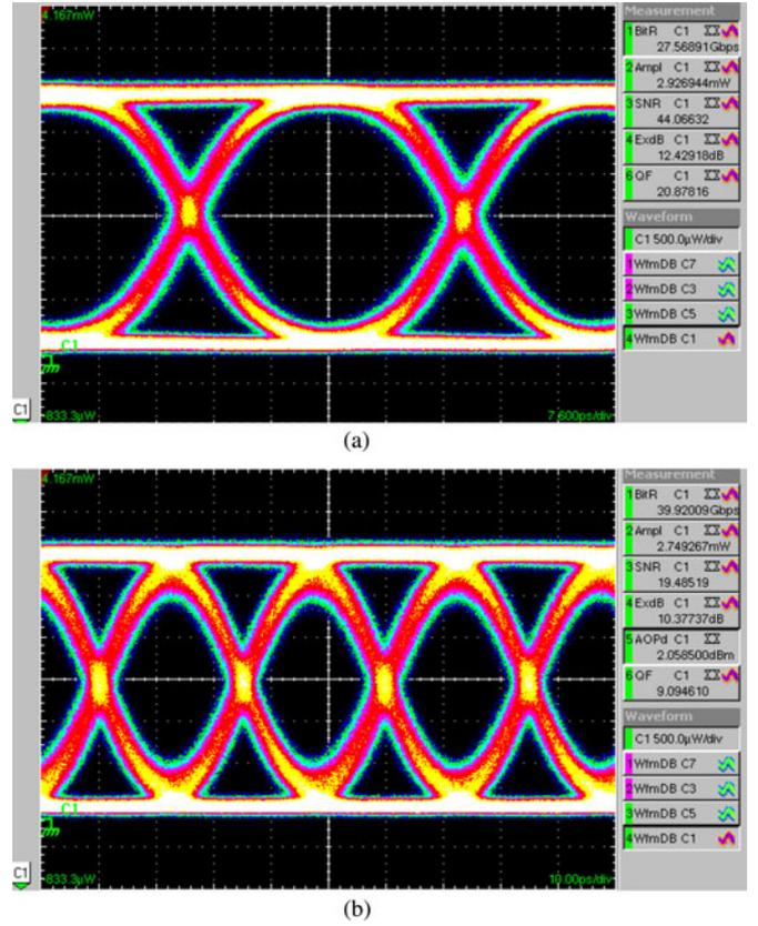
Fig. 9. Si TWMZ extinction measurement: (a) 12.4 dB extinction at 28 Gb/s and (b) 10 dB extinction at 40 Gb/s.
