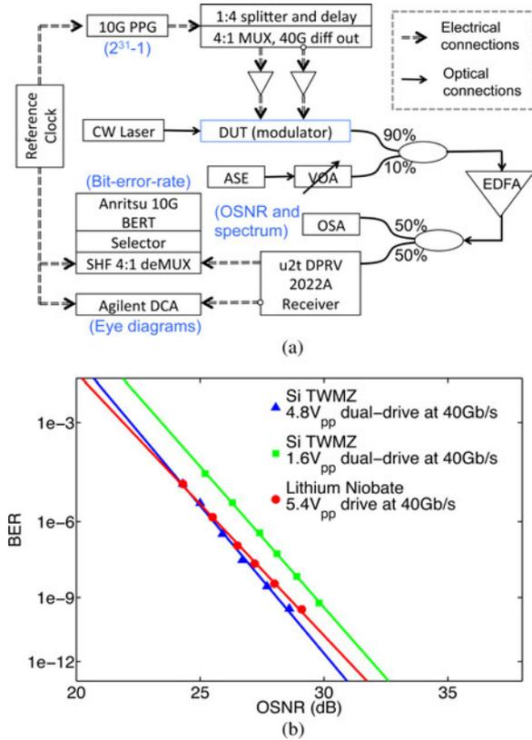
Fig. 7. (a) Experiment setup for BER and eye-diagram measurements (PPG: pulse pattern generator, OSA: optical spectrum analyzer, VOA: variable optical attenuator, ASE: amplified spontaneous emission). (b) BER versus OSNR.
