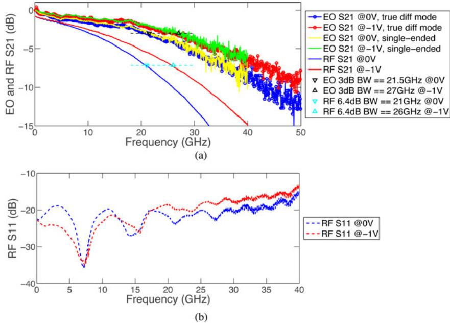
Fig. 6. EO and RF S-parameters at 0 and  $-1$  V bias. (a) EO and RF S21. (b) RF S11.
