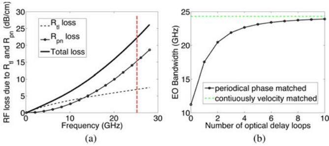
Fig. 4. (a) Simulated RF loss due to p-n junction series resistance  $R_{pn}$  and transmission line metal resistance  $R_{tl}$ , red dashed line marks the 3-dB bandwidth location, and (b) Simulated EO bandwidth versus numbers of optical delay loops, the green dashed line marks the 3-dB bandwidth of a continuously velocity matched modulator that has the same RF loss.
