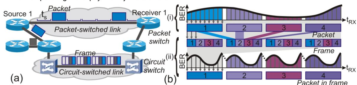
**Fig. 1:** (a) Packet-switched and circuit-switched networks; (b) mapping of BER variations onto bit errors within a packet (i), and time compression of BER variations when splitting a packet across multiple TDM frames (ii).
