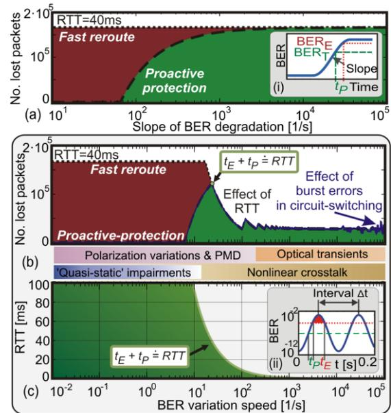
**Fig. 2:** Number of lost packets (dotted: FRR, dashed: PPT) vs. (a) slope of BER step (i), and (b) BER variation speed  $1/\Delta t$  (ii); (c) Region where PPT outperforms FRR.
