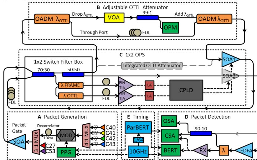
Fig. 1 Experimental Setup Diagram
