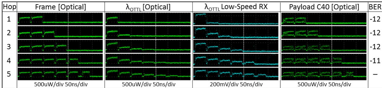
Fig. 3 CSA screen-capture of Frame,  $\lambda_{OTTL}$ , Low-Speed PIN-TIA, and Payload Channel for 1-5 Hops
