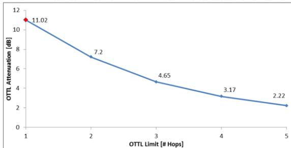
Fig. 4 OTTL Attenuation for 1-5 hops
