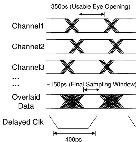
**Figure 14.** Effect of cumulative channel skew relative to the source synchronous clock.
