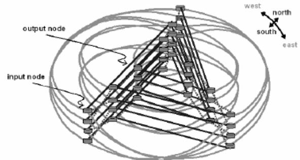
**Figure 1.** Optical Packet Switching Network (12x12 Data Vortex) [6].
