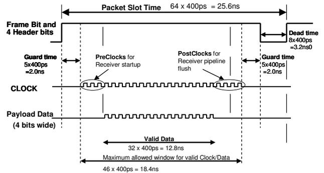
**Figure 3.** Test stimuli signals needed for the Optical Test Bed application [10].
