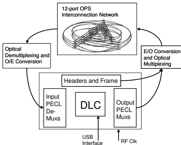
**Figure 2.** Optoelectronic test application (Data Vortex).
