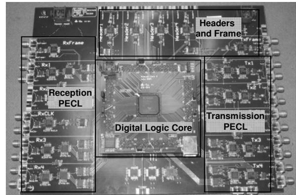
**Figure 6.** Transmitter and Receiver electronics used for the Optical Test Bed application.
