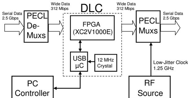
**Figure 4.** Using a programmable Digital Logic Core with high-speed PECL for testing an optical network.
