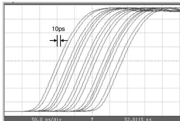
Figure 9. Time shifted signal in 10ps (programmed) steps.
