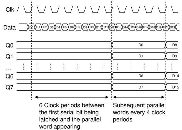
**Figure 12.** Signal timing of the deserialization process.
