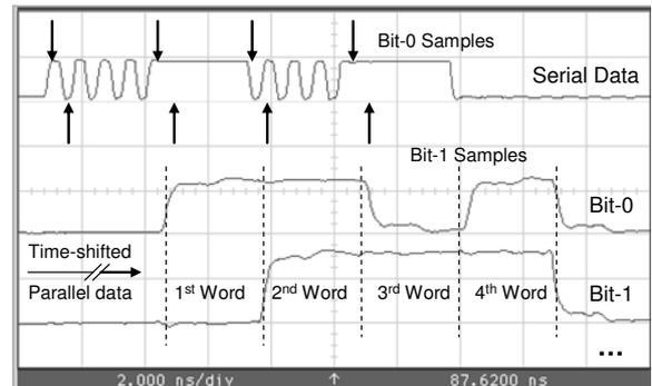
**Figure 13.** Demultiplexed serial data stream.
