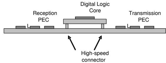
**Figure 5.** Cross-section view of Optical Test Bed electronics.
