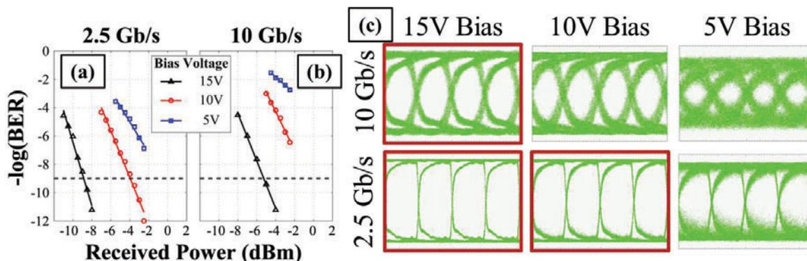
Fig. 2. BER curves for (a) 2.5 Gb/s and (b) 10 Gb/s, (c) electrical eye diagrams taken after the TIA-LA for 2.5 Gb/s and 10 Gb/s data at 15V, 10V and 5V detector bias. Error-free eyes are shown with red outline.
