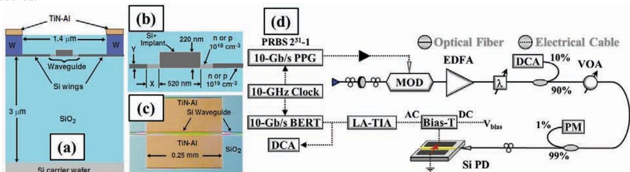
**Fig. 1.** (a) Cross-Section of a Si<sup>+</sup> ion implanted Si PIN PD, (b) close up of (a) with WG measurements and doping profiles, (c) top-view optical microscope image, (d) experimental setup. (a)-(c) reprinted from [5].
