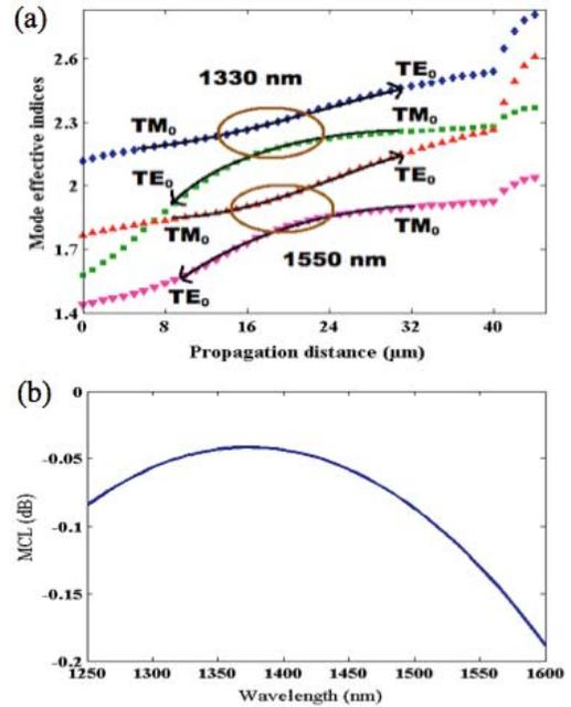
Fig. 2. (a) Mode effective indices evolution along the PSR structure. (b) Simulated MCL of the bi-level taper.
