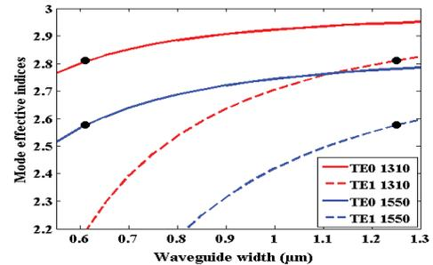
Fig. 3. Effective indices of the TE<sub>0</sub> mode and the TE<sub>1</sub> mode at 1310 nm and 1550 nm as a function of waveguide width.
