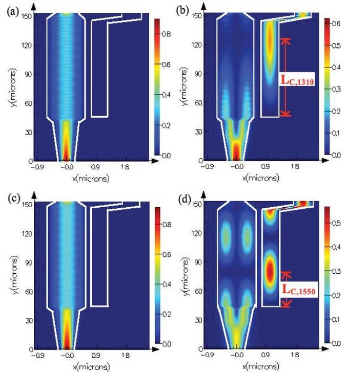
Fig. 5. Mode propagation when launching (a)  $TE_0$  at 1310 nm, (b)  $TM_0$  at 1310, (c)  $TE_0$  at 1550 nm, and (d)  $TM_0$  at 1550 nm.
