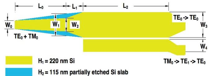
Fig. 1. Schematic of the proposed bi-wavelength PSR with significant geometric parameters noted.
