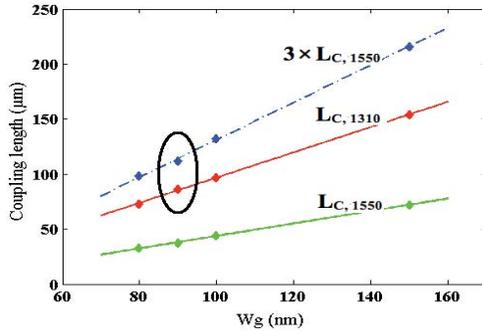
Fig. 4.  $L_{C,1310}$  and  $L_{C,1550}$  as a function of  $W_g$ .
