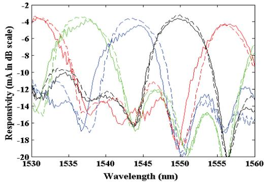
Figure 3. Spectra of four channels at (a) the lowest-loss polarization state (dashed line) (b) the highest-loss polarization state (solid line).
