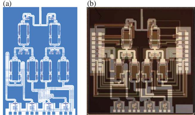
Figure 1. (a) Layout of the receiver chip without showing the metal wire and pads that are used to bias the MZIs. (b) Chip photo.
