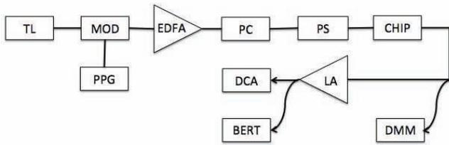
Figure 2. Experiment setup for performance evaluation.
