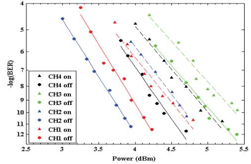
Figure 5. Experimental results of BER measurements at 10 Gbps. Dashed and solid lines represent when the scrambler is on and off, respectively.
