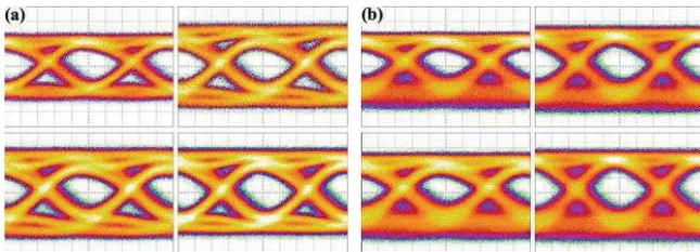
Figure 4. Received electrical eye from all channels at 40 Gbps (a) without (b) with scrambled polarization (3 mV/div, 5 ps/div).
