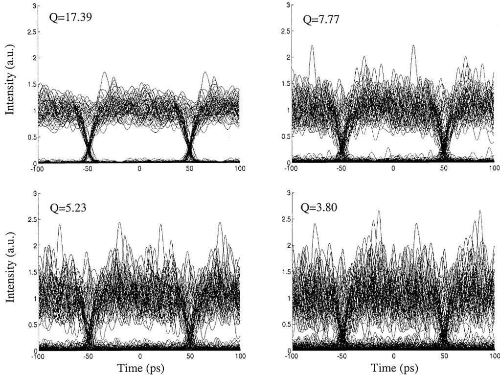
**Figure 5.** Evolution of the eye diagram for five WDM channels spaced 2 nm apart over 12 cascaded SOAs (nodes). The transmission penalties at each node are derived from (1) with the parameters fit to Fig. 3. Note that this is only a single realization of the data and noise.
