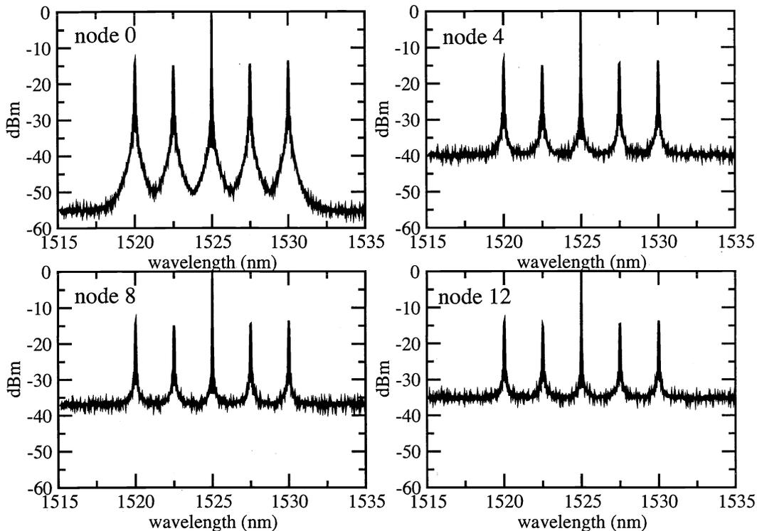
**Figure 4.** Evolution of the spectrum of five WDM channels spaced 2 nm apart over 12 SOAs (nodes). The transmission penalties at each node are derived from (1) with the parameters fit to Fig. 3. Two hundred realizations have been simulated.
