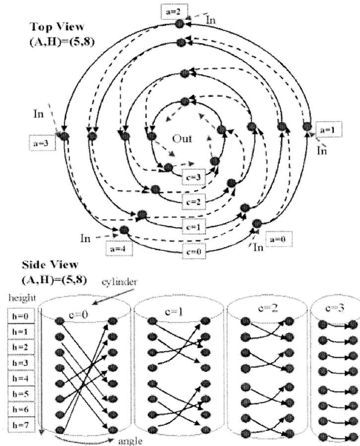
**Figure 1.** Data Vortex topology with the parameters  $(A, H) = (5, 4)$  and nodes labeled by  $(a, c, h)$  where  $0 < a < A, 0 \leq c < C$  and  $0 \leq h < H$ . The routing tours are seen from the top and side. Information is input on the outermost cylinder ( $c = 0$ ) and is propagated to the appropriate output port on the innermost cylinder ( $c = C - 1$ ).
