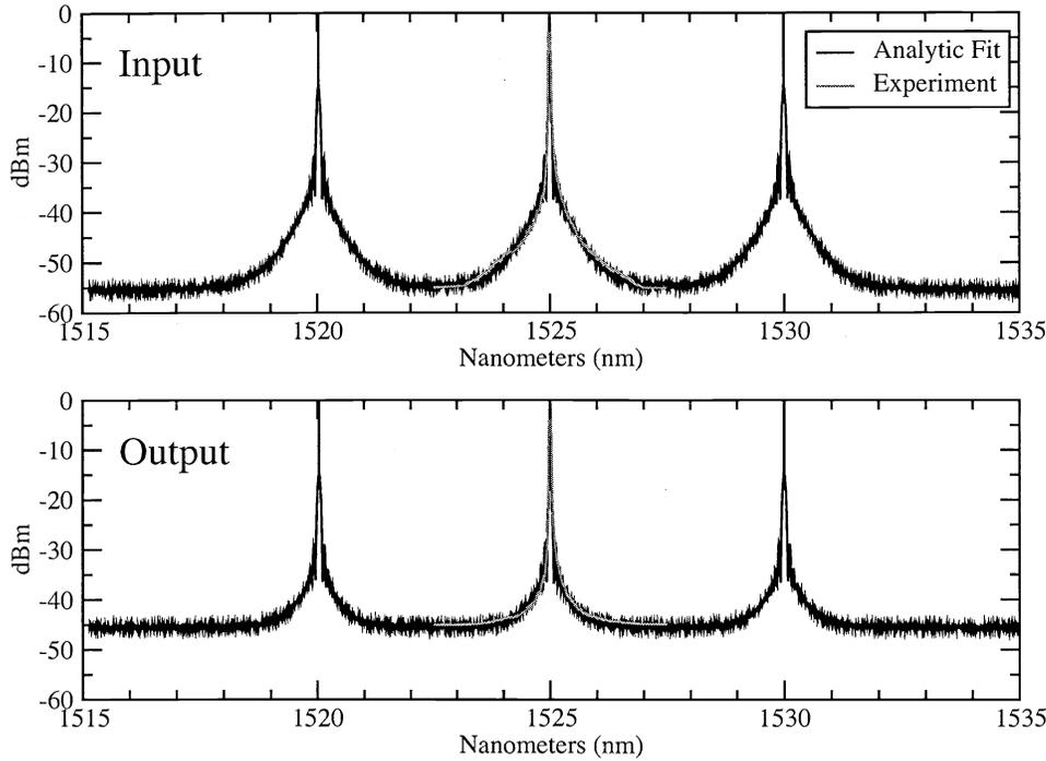
**Figure 3.** Analytic fit, using  $A$ ,  $B$ , and  $C$ , to the experimentally measured noise penalties due to white-noise and a Lorentzian contribution. The analytic data corresponds to (1) where 500 realizations have been averaged over. Three channels have been used in the experimental fit with a channel spacing large enough so that no noticeable overlap occurs between neighboring Lorentzian contributions.
