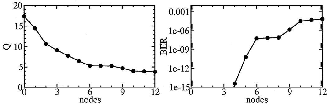
**Figure 6.** Q factor and BER for five WDM channels spaced 2 nm apart over 12 cascaded SOAs (nodes). The transmission penalties at each node are derived from (1) with the parameters fit to Fig. 3. Note that this is only a single realization of the data and noise.
