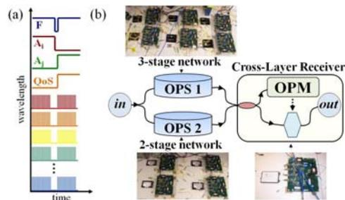
Fig. 2: (a) Packet format; (b) Block diagram and photographs of fabric test-bed with cross-layer scheme
