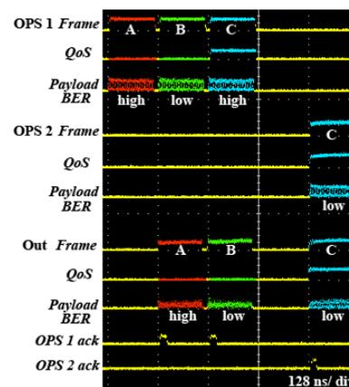
Fig. 3: Input and output optical waveforms of the experimental packet sequence (colours refer to different time-division multiplexed packet streams)
