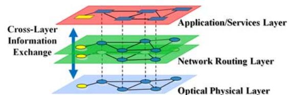
Fig. 1: Cross-layer optimized protocol stack
