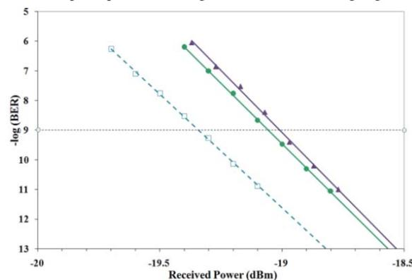
Fig. 4. BER sensitivity plots for one wavelength channel ( $\lambda=1559.7$  nm) recorded without the multipulse pre-emphasis signal (purple,  $\blacktriangle$ ), with the multipulse signal (green,  $\bullet$ ), and the back-to-back signal (blue,  $\square$ ).
