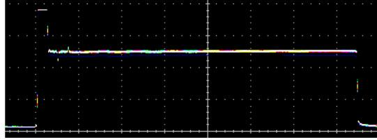
Fig. 1. The implemented multipulse current injection pulse for reducing the SOA turn-on response time.
