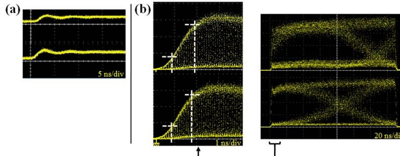
Fig. 3. [top: without pre-emphasis current injection, bottom: with pre-emphasis current injection] (a) Rise time of a single CW signal; (b) Waveforms of one 10 Gb/s channel of the 150-ns optical packet with magnified views of the rising edge: dashed lines show the 20/80 rise time.
