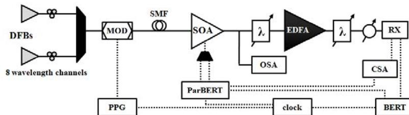
Fig. 2. Experimental setup used to determine BER performance. Solid lines indicate optical fiber, while dashed lines indicate electrical cable.
