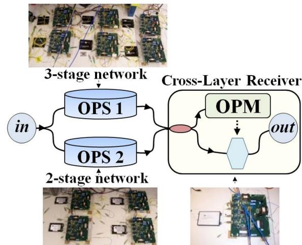
Figure 3. Diagram and photographs of the optical network test-bed with customized cross-layer enabled receiver design [7].
