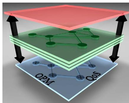
Figure 1. Envisioned cross-layer-optimized network stack, with OPM devices embedded in the physical layer.
