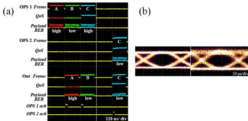
Figure 4. (a) Optical waveforms, with colours pertaining to the different time-multiplexed packet streams; (b) 10-Gb/s input (left) and output (right) eye diagrams [7].
