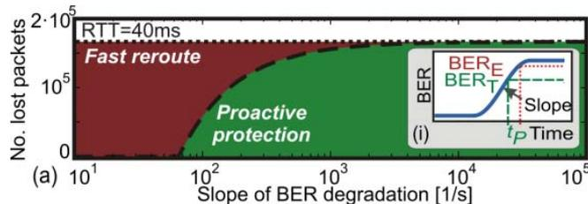
Figure 2. Simulated comparison of packet loss performance between fast-reroute and proactive packet protection mechanisms [5].
