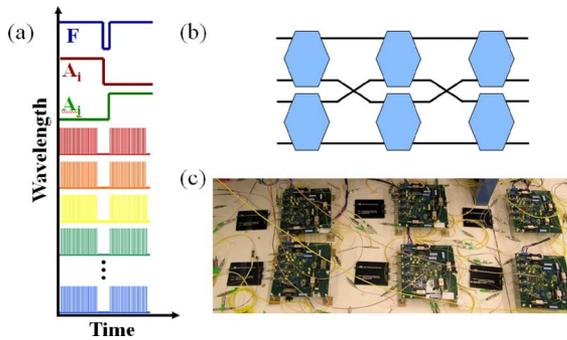
Fig. 1. (a) Wavelength-striped optical packet format. (b) Network block diagram. (c) Photograph of implemented network test-bed.
