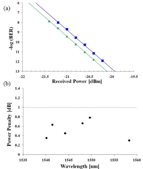
Fig. 4. (a) 10-Gb/s sensitivity curves for one representative wavelength ( $\lambda = 1558.28$  nm) [ $\blacktriangle$  back-to-back;  $\blacksquare$  through]. (b) Power penalty with respect to all six payload wavelength channels.
