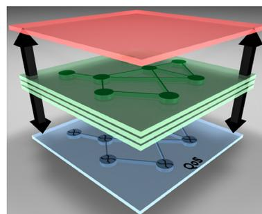
**Fig. 1:** Cross-layer-optimized stack, indicating the bidirectional information flow between the application (top), network and routing (middle), and optical layers (bottom) enhanced to provide QoS guarantees.
