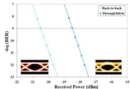
Fig. 6: Sensitivity curves with insets of the 10-Gb/s eye diagrams (input: left, output: right).
