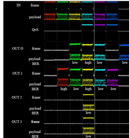
Fig. 5: Optical waveforms corresponding to the QoS-aware packet multicasting operation.
