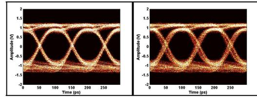
Fig. 4: 10-Gb/s TiSER-generated eye diagrams pertaining to packets at the network input (left) and output (right) ( $\lambda=1556.6$  nm).
