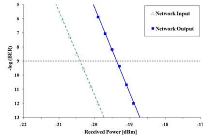
Fig. 5: BER curves ( $\lambda=1556.6$  nm) for the test-bed.
