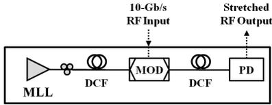
Fig. 2: Physics of the time-stretch pre-processor.
