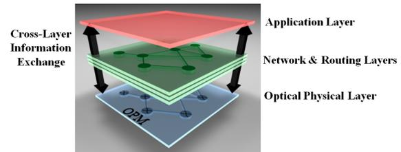
**Fig. 1:** OCL stack, depicting the bidirectional information flow between the application (top), network and routing (middle), and optical layers (bottom) with embedded OPM devices.
