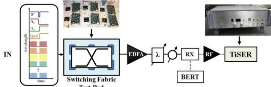
Fig. 3: Block diagram and photographs of the experimental demonstration with the optical fabric test-bed and TiSER.
