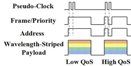
Fig. 2. Diagram depicting the implemented OQoS encoding scheme for the supported wavelength-striped optical packet.
