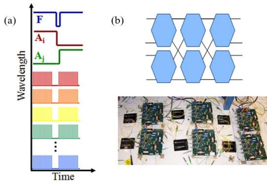
Fig. 1. (a) Wavelength-striped optical message structure, depicting the optical packet header signals, such as the frame (F) and address bits ( $A_i$ ,  $A_j$ ), and modulated payload wavelength channels; (b) three-stage switching fabric network topology and test-bed photograph.
