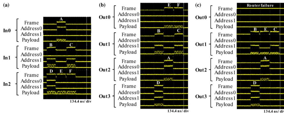
Fig. 2. Optical waveform traces of the experimental packets taken at the (a) fabric input; (b) fabric output under an online router scenario with all output ports functional; (c) fabric output in the case of an offline router, with switching fabric aware that link out0 is down/degraded.
