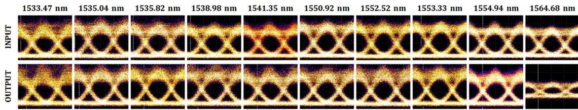
Fig. 3. A 10-Gb/s optical eye diagrams for the input and output of the switching fabric, for all ten payload wavelength channels.
