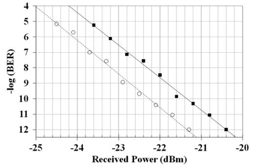
Fig. 4. Sensitivity curves for one payload channel ( $\lambda = 1564.68$  nm). The dashed line with open points corresponds to the back-to-back measurements, while the solid line with filled points refers to the data at the fabric's output.
