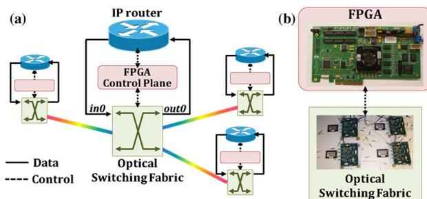
Fig. 1. (a) Envisioned network architecture with network nodes composed of IP routers, optical packet switching fabrics, and an FPGA-based control and management plane. The FPGA acts as a cross-layer interface, accepting control inputs to manage physical-layer switching. (b) Photographs of FPGA circuit board and implemented OPS fabric used in this demonstration.
