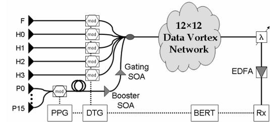
**Fig. 2:** Experimental setup consisting of lasers (black triangles), a pulse pattern generator (PPG), a data timing generator (DTG), LiNbO<sub>3</sub> modulators (mod), a decorrelator (loops), SOAs (grey triangles), a coupler (oval), a tuneable filter ( $\lambda$ ), an EDFA, a receiver (Rx), and a BER tester (BERT).
