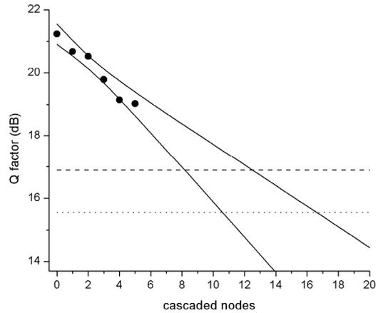
**Fig. 4:** Plot of a packet's Q factor as a function of the number of nodes through which it has propagated. Solid lines represent the minimum and maximum projected Q factors based on a linear curve fit. The dashed and dotted lines signify BERs of  $10^{-12}$  and  $10^{-9}$  respectively.
