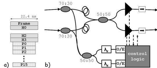
**Fig. 1:** Switching fabric (a) packet structure and (b) transparent node design. The node consists of couplers (ovals with splitting ratios), filters ( $\lambda$ ), PIN-TIAs (O/E), electronic control logic, fibre delay lines (loops), SOAs (triangles), and isolators (arrows). Optical and electrical connexions are shown with solid and dashed lines respectively.
