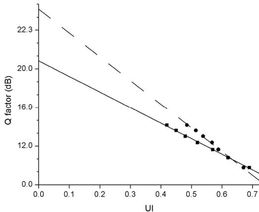
**Fig. 3:** Extrapolation of Q factor for time (solid) and amplitude (dashed) measurements after two data vortex nodes. (A linear extrapolation was performed on the Q factor and plotted in logarithmic units.)
