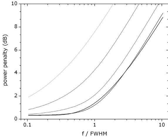
**Fig. 2.** Power penalty as a function of the bit rate,  $f$ , normalized to resonator FWHM for optical signals after passing through a microring. From heaviest to lightest, the contours represent the NRZ, and the 33%-, 10%-, 3%-, and 1%-RZ data formats.
