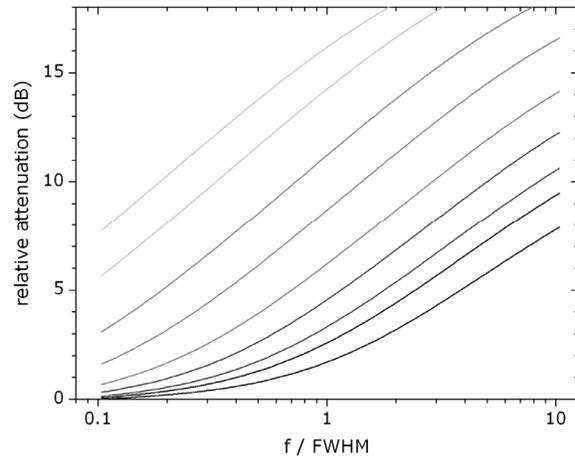
**Fig. 3.** Relative signal attenuation due to sideband distortion versus bit rate,  $f$ , normalized to resonator FWHM for optical signals after passing through a microring. From heaviest to lightest, the contours represent the NRZ, and the 67%-, 50%-, 33%-, 20%-, 10%-, 5%-, 2%-, and 1%-RZ data formats.
