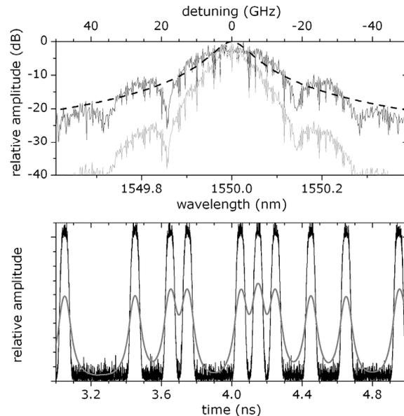
**Fig. 1.** (a) Modulation spectra and (b) time domain representations of 10 Gbps 50%-RZ optical signals, shown before (black) and after (gray) passing through a microring, modeled by a Lorentzian (dashed) with a  $Q$  factor of 20,000 (FWHM of 10 GHz).
