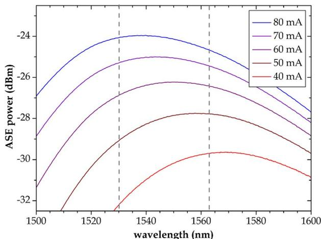
Fig. 4. ASE spectra taken for the Alcatel SOA at varying drive current levels with no optical input. The dashed lines indicate the wavelength band used throughout this study.
