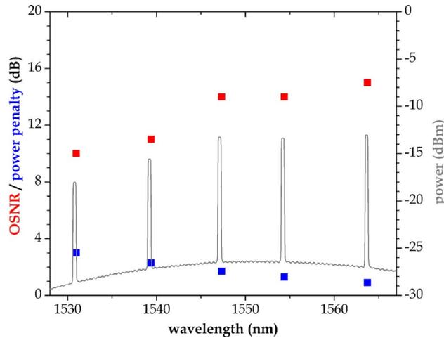
Fig. 8. Power penalty, OSNR, and spectral power with SOA operation lower than the optimized current. Average power penalty is 1.8 dB, and gain variance is 5.0 dB.
