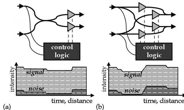
Fig. 2. Schematic (top) and packet power diagram (bottom) of the (a) single packet and (b) nonblocking SOA-based OPS nodes. The optical power can ideally be preserved through the node with only slight additions in noise power. However, the wavelength-dependent gain–loss limits this desired property.
