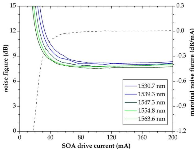
Fig. 6. Noise figure (solid curves) plotted against drive current for each of the five wavelength channels that simultaneously propagate through the SOA with packet input power of -11 dBm. The marginal noise figure (dashed curve) is the numerical derivative of the average noise figure over the five wavelengths.
