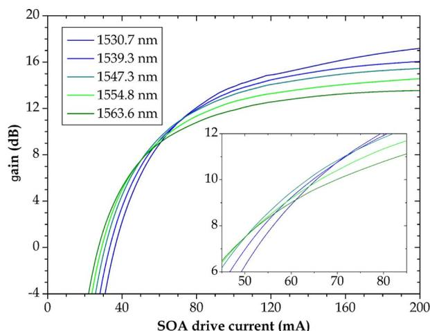
Fig. 3. Gain versus drive current for the Alcatel SOA for the five-wavelength signal with a total packet input power of  $-13$  dBm. The inset zooms in on the optimal operating point.
