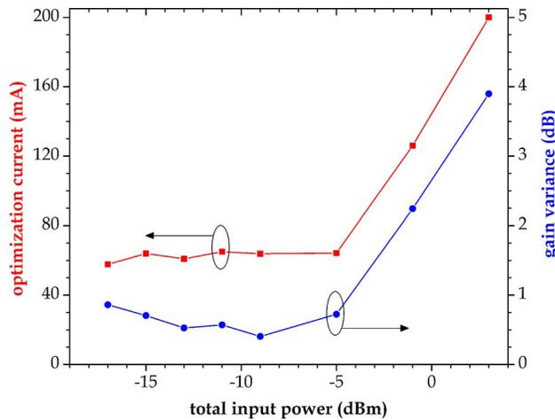
Fig. 5. Input power characteristics of the gain-variance-optimized operating point. The left axis (■) plots the drive current required to minimize gain variance. The right axis (●) plots the measured SOA gain variance at a constant drive current of 62 mA.
