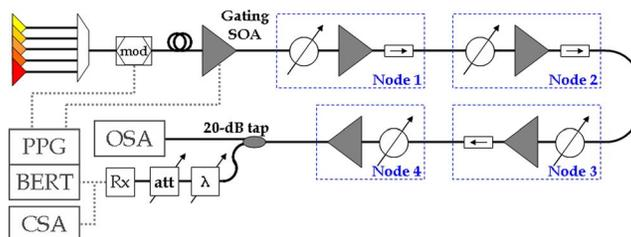
Fig. 7. Experimental setup including a multiple-wavelength packet transmitter, a cascade of four nodelike structures, a receiver, and test and measurement equipment.
