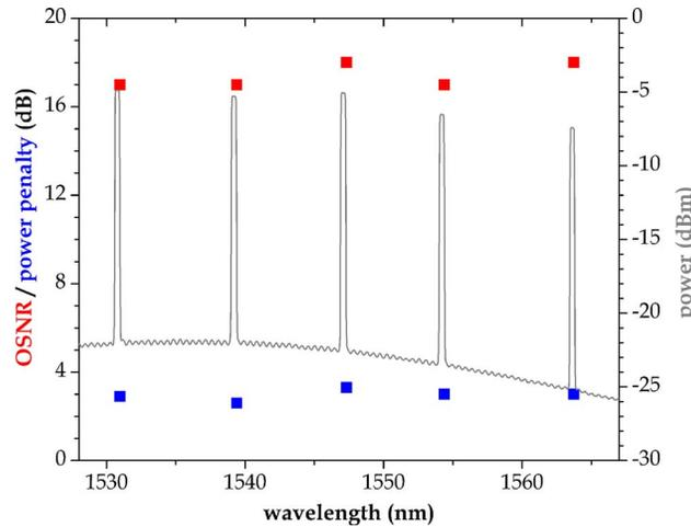
Fig. 10. Power penalty, OSNR, and spectral power with SOA operation higher than the optimized current. Average power penalty is 3.0 dB, and gain variance is 2.5 dB.
