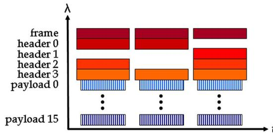
Fig. 1. Example of a multiple-wavelength packet format. This specific format utilizes 16 payload channels alongside five single-bit routing channels [11–13].
