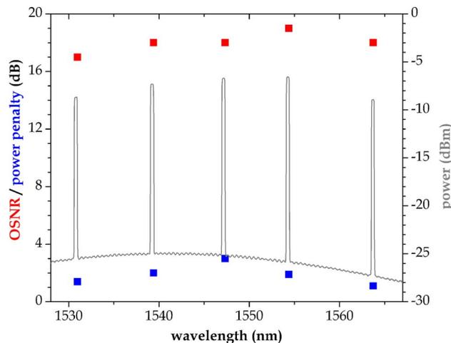
Fig. 9. Power penalty, OSNR, and spectral power with SOA operation at the optimization current. Average power penalty is 1.9 dB, and gain variance is 2.3 dB.
