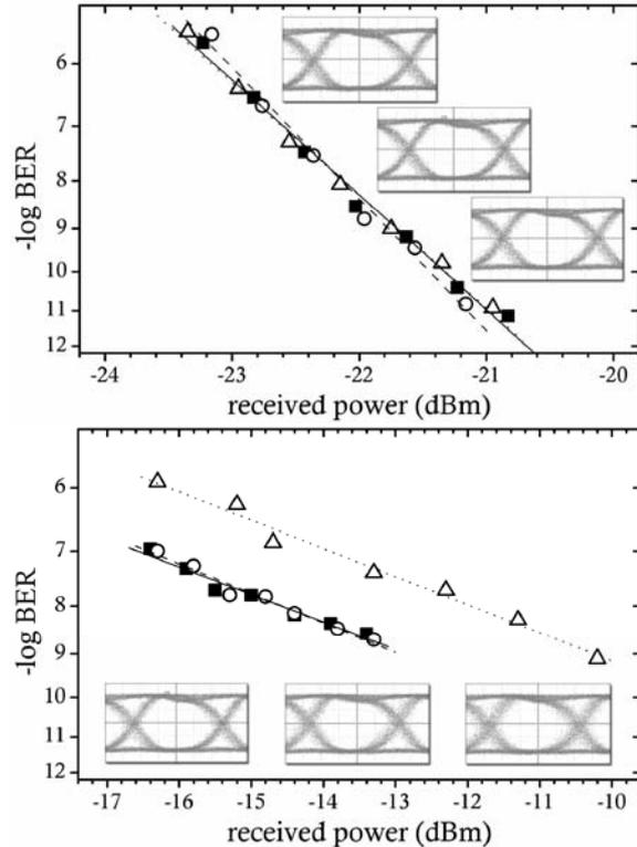
Fig. 3. BER curves for TM (top) and TE (bottom) modes exiting ports A (■), B (○), and C (Δ) with inset eye diagrams from A (left), B (center), and C (right).
