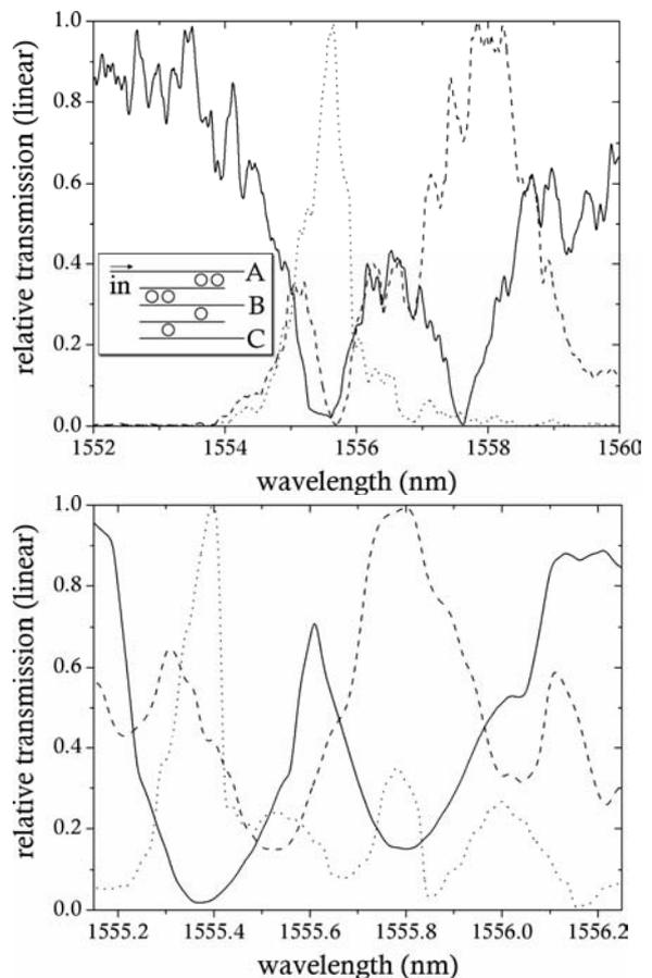
Fig. 1. Transmission spectra of three TM-mode (top) and TE-mode (bottom) outputs: A (solid), B (dashed), and C (dotted), with schematic inset in upper plot.
