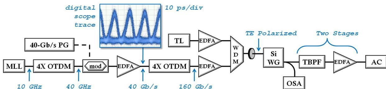
Fig. 1. Experimental setup consisting of a mode-locked fiber laser (MLL), optical time-division multiplexers (OTDM), pattern generator (PG), LiNbO<sub>3</sub> modulator (mod), tunable laser (TL), erbium-doped fiber amplifiers (EDFA), wavelength-division multiplexer (WDM), fiber polarizer, silicon waveguide (Si WG), optical spectrum analyzer (OSA), tunable bandpass filters (TBPF), and autocorrelator (AC). The inset shows a 40-Gb/s RZ eye diagram following the optical modulator and EDFA.
