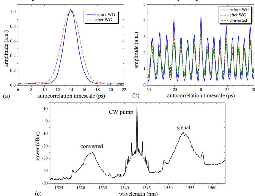
Fig. 2. (a) Autocorrelator traces recorded for a picosecond pulse before and after injection into the waveguide, without wavelength conversion. (b) Autocorrelator traces taken on a 160-GHz pulse train before and after injection into the waveguide without wavelength conversion, and also after injection into the waveguide with wavelength conversion. (c) OSA trace displaying the spectrum immediately following the waveguide, demonstrating wavelength conversion of a 160-Gb/s data signal.
