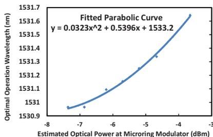
**Fig. 4:** Optimal operation wavelength with varied optical power.
