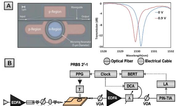
**Fig. 1:** (a) Scanning-electron-microscope (SEM) image and spectrum of the microring modulator. (b) Experimental Setup.
