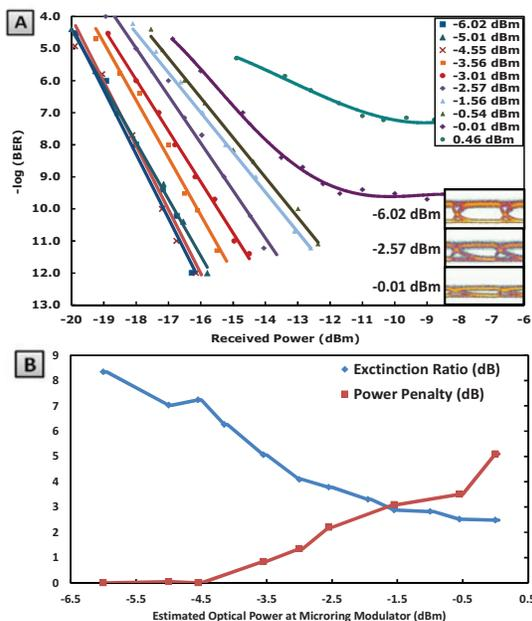
**Fig. 3:** (a) Recorded BER curves with increasing optical power at fixed wavelength, legend shows estimated optical power at microring modulator. (b) Extinction ratio and power penalty vs. estimated optical power.
