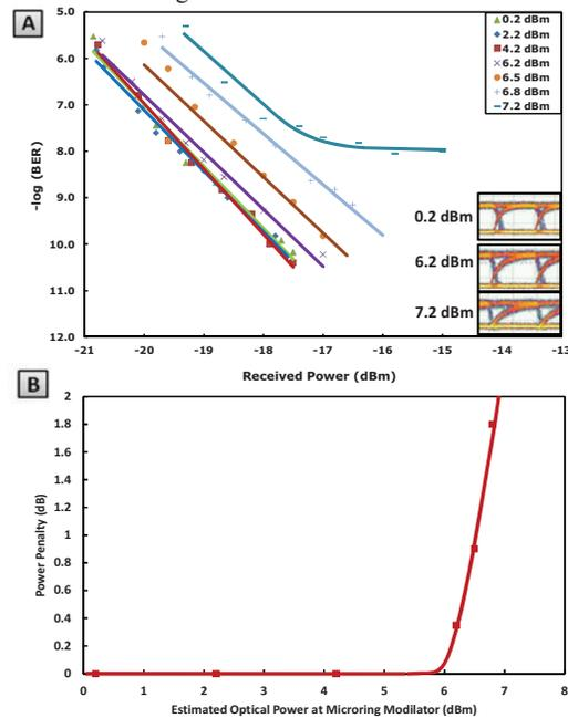
**Fig. 5:** (a) Recorded BER curves with increasing optical power at tuned modulation bias. (b) Power penalty vs. estimated optical power.
