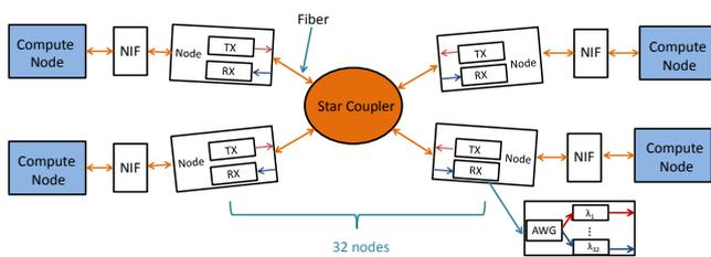
**Figure 3.** Optical Network Architecture in PhoenixSim
