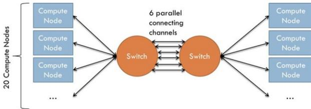
**Figure 2.** Layout of Electrical Baseline Simulation Model
