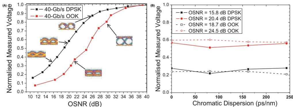
Fig. 4. (a) Normalized measured photodiode voltage as a function of OSNR. Insets: eye diagram of the 40-Gb/s OOK and demodulated DPSK signals. (b) Normalized measured photodiode voltage as a function of chromatic dispersion with different OSNR.
