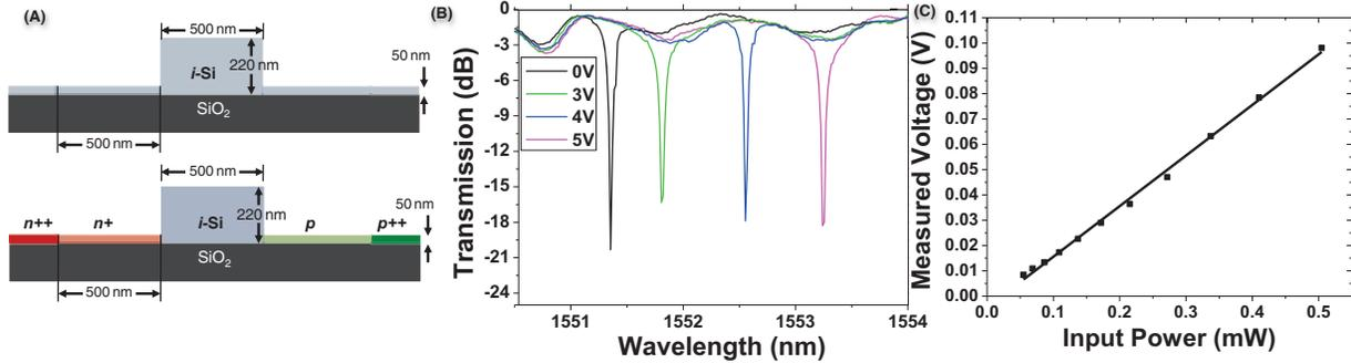
Fig. 2. (a) Waveguide geometry and doping profile for the microring (top) and silicon photodiode (bottom). (b) Transmission spectra of the microring at different heater voltages. (c) Measurement of the silicon photodiode linearity.
