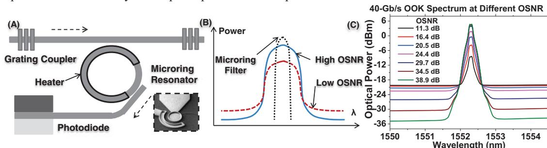
Fig. 1. (a) The OSNR monitor, composed of a microring resonator with integrated heater and silicon photodiode positioned on the drop port of the microring (not to scale). Inset: SEM image of fully processed device. (b) Working principle of the OSNR monitor. (c) Measured 40-Gb/s OOK spectrums at various OSNR.
