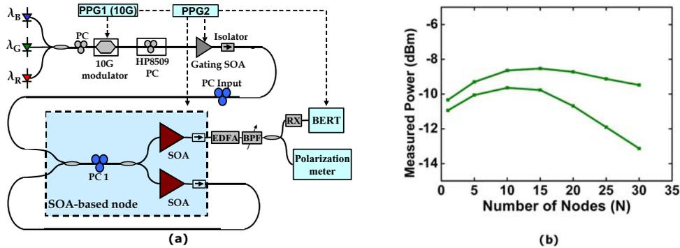
Fig.1. (a) Re-Circulating Loop. PPG: pulse pattern generator; SOA: semiconductor optical amplifier; EDFA: erbium doped fiber amplifier; BPF: bandpass filter; RX: optical receiver module; PC Input: polarization controller to change input SOP; PC 1: polarization controller to change node PDG. Optical path (solid line); Electrical path (dashed line). (b) Minimum and maximum power for various input SOPs measured at channel  $\lambda_G$  (1543 nm) with maximized PDL in the loop.
