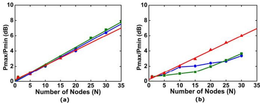
Figure 2: (a) Maximized PDG for  $\lambda_G$  (green) with corresponding PDG on  $\lambda_B$  (blue), and  $\lambda_R$  (red) (PC1 setting is the same for each wavelength). (b) Maximum cascaded PDG for  $\lambda_B$  (blue),  $\lambda_G$  (green) and  $\lambda_R$  (red) (PC1 setting is different for each wavelength).
