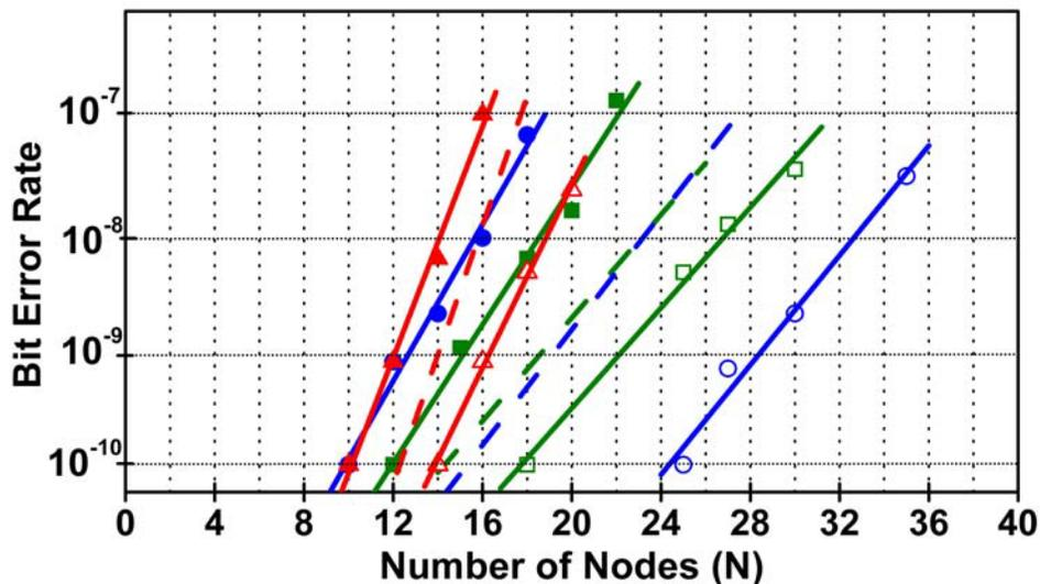
Fig. 3. BER measurements on all three payload channels (blue circles: 1531 nm; green squares: 1543 nm; red triangles: 1553 nm).
