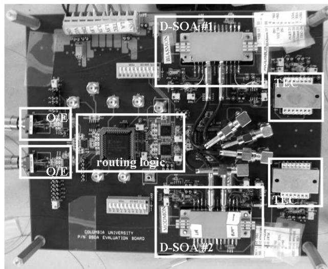
Fig.5. Optimized SOA-based switching node with two temperature-controlled D-SOA devices, optical receiver (O/E) and routing logic.
