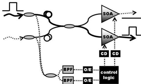
Fig. 3: Switching node configuration of the data vortex network with a single packet being routed through one output port (BPF: optical bandpass filter, O/E: optical-to-electrical conversion, CD: current driver).
