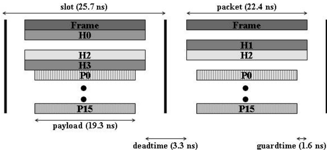
Fig. 2. Packet structure: payload and routing headers encoded on DWDM channels.
