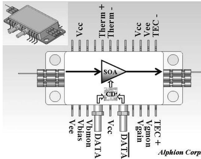
Fig. 4. D-SOA pin-out. Modified 28-pin butterfly package with two sub-SMB connectors (inset).
