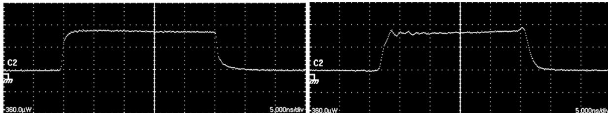
Fig. 6. Optical signal at the output of the D-SOA (left) and of a commercial SOA (right).
