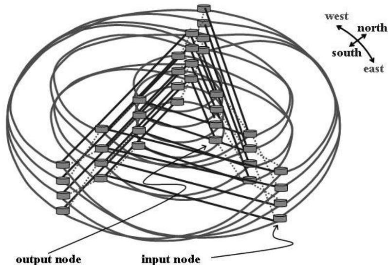
Fig. 1. Data vortex topology corresponding to a 12-port interconnection network that contains 36 switching nodes.
