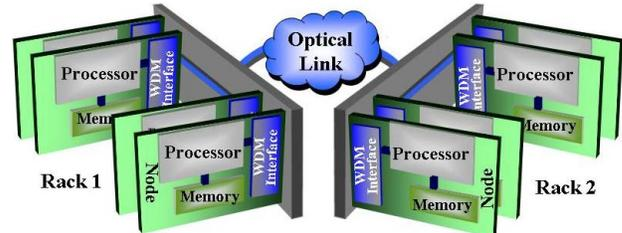
Fig. 1 Transparent WDM interface for inter-node communication infrastructure.
