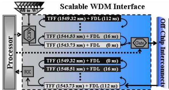
Fig. 2: Schematic of the WDM interface for off-chip.
