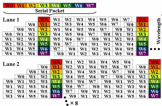
Fig. 3: Serial electronic packets onto multiple WDM channels.
