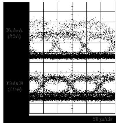
Fig. 5 Eye diagrams at switch output (south) from payload channel at  $\lambda_5=1553.3\text{nm}$ . Upper trace represents output from node A (SOA gate) and lower trace represents output from node B (LOA gate).
