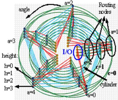
Fig. 1 Schematic of the Data Vortex topology with  $A=5$ ,  $H=4$ . The routing nodes are interconnected on  $C=3$  concentric cylinders.
