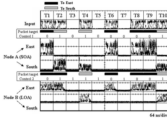
Fig. 4 Routing results at node A (SOA) and node B (LOA) from payload channel at  $\lambda_5=1553.3\text{nm}$ . A similar result is obtained from payload channel at  $\lambda_4=1545.3\text{nm}$ .
