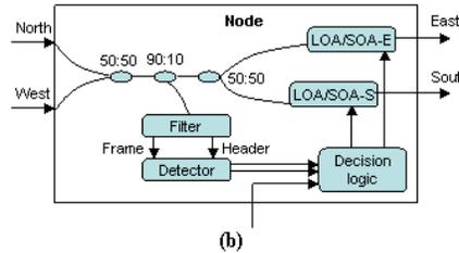
Fig. 3 (a) Two-node WDM routing test-bed schematic. (b) Routing node structure. PPG: pulse pattern generator; LD: laser diode; EDFA: Erbium doped fiber amplifier; LOA: linear optical amplifier; SOA: semiconductor optical amplifier.
