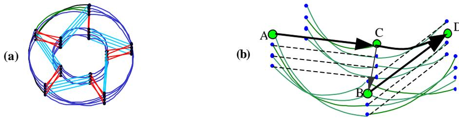
Fig.1. (a) Schematic of the Data Vortex topology with 2 cylinder and 5 angles. (b) Demonstrated Data Vortex sub-system. The large solid circles are the experimentally constructed nodes. The arrow from C to B indicates the control signal path. The arrows from A to C, C to D, and B to D are data paths.
