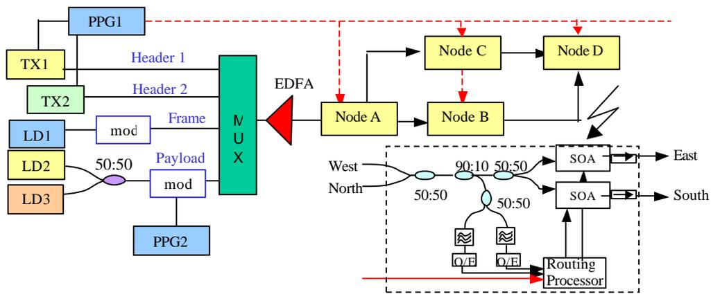
Fig. 2. Four-node routing test-bed schematic and node structure. PPG: pulse pattern generator; TX: transmitter; LD: laser diode; EDFA: Erbium doped fiber amplifier; SOA: semiconductor optical amplifier.
