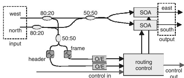
Fig. 1 Data vortex switching node structure
