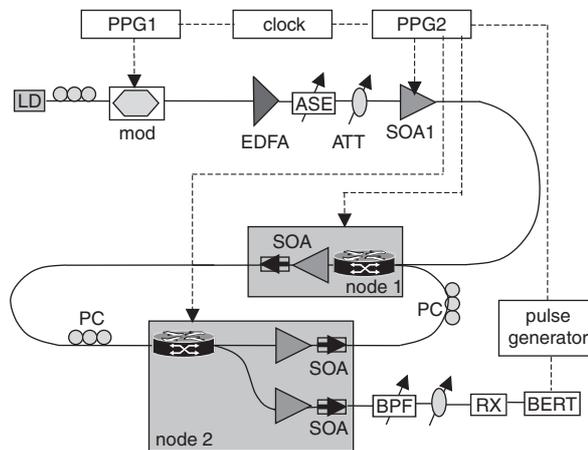
Fig. 2 Experimental setup of switching-loop test-bed
