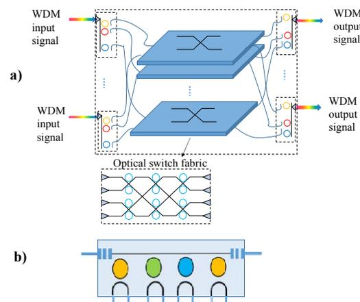
**Fig. 1 a)** OXC architecture with microring based wavelength selective filters at the input, spatial switches and multiplexors **b)** ROADM device architecture with microrings.
