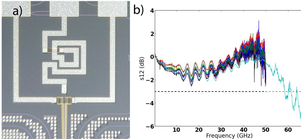
Figure 3. a) Image of the Germanium photodetector showing the inductive gain peaking element. b) EO response of a large number of detectors up to 50 GHz and a single measurement showing a 58 GHz bandwidth.
