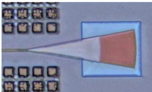
Figure 2. Image of a platform grating coupler. The gratings are in the dark red region.
