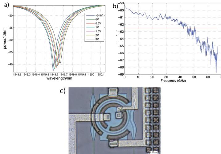
Figure 4. a) Resonance peaks of the ring resonator at various bias voltages. b) EO bandwidth at 0 V bias showing a 3 dB bandwidth of 45 GHz. c) Image of a ring resonator showing the ring, input waveguides and metal wiring.
