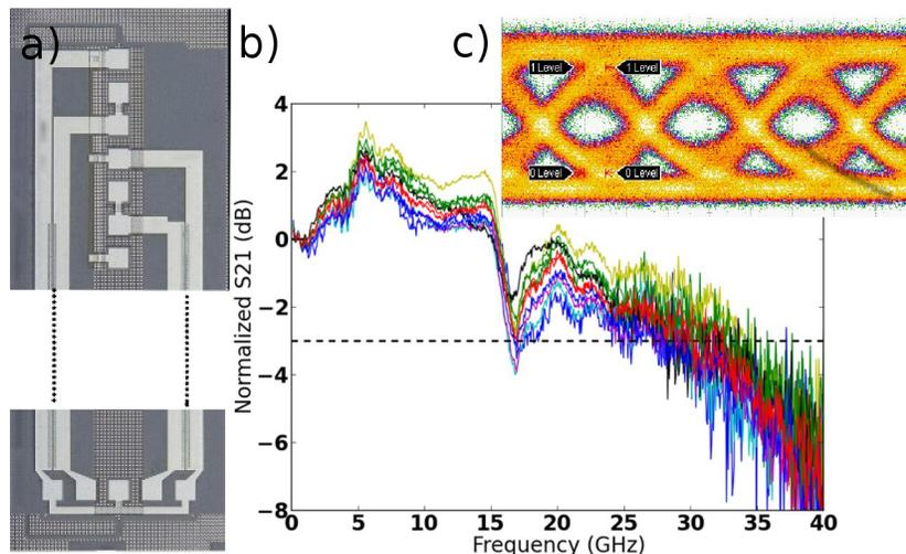
Figure 5. a) Image of the traveling wave Mach-Zehnder. b) RF response of a number of modulator arms showing a typical 3 dB bandwidth of 30 GHz. c) Eye diagram at 40 Gb/s with differential drive voltage of 2.5 Vpp.
