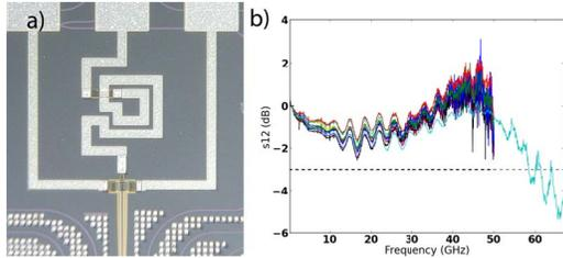
**Figure 2.** a) Image of gain-peaked photodetector. b) EO response of a number of photodetectors up to 50 GHz and a single high-speed measurement showing 58 GHz bandwidth.
