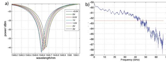
**Figure 4.** a) Ring resonance shift at different bias voltages. b) EO response at 0 V bias showing a 3 dB bandwidth of 45 GHz.
