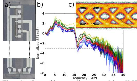
**Figure 3.** a) Image of 3mm traveling wave modulator. b) RF performance of a number of modulator arms at 1V bias. The amplitude shows a typical 3 dB bandwidth of 30 GHz. c) Eye diagram at 40 Gb/s with differential drive voltage of 2.5 Vpp.
