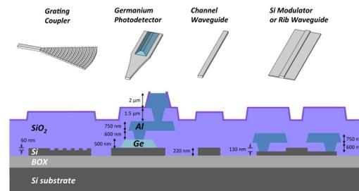
Figure 1. Illustration of the platform cross-section
