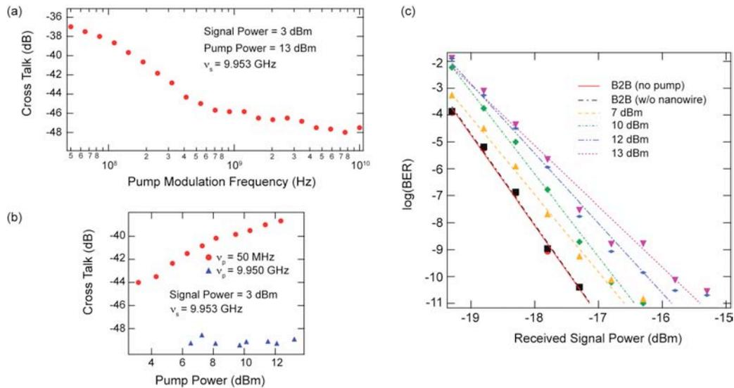
Fig. 1. Experimental results. (a) Crosstalk as a function of pump modulation frequency. (b) Crosstalk as a function of pump power. (c) BER measurement for various signal powers. The numbers represent the power inside the nanowaveguide. Two back-to-back measurements are performed, one with no pump and the other with the nanowaveguide removed from the setup.
